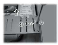
3. Push the power fixture bracket completely to hold the power supply, and then affix the interface card bracket by screws (A, B, C)
