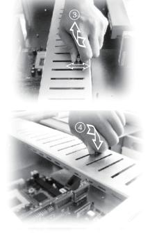
3. Loose the thumb screws to adjust the hold down clamp to the interface card
