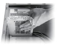
1. Place the power supply into the case
