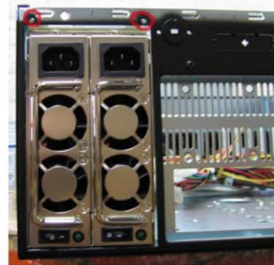
8. Fix the PSU with two additional screws in the rear (marked spots)
