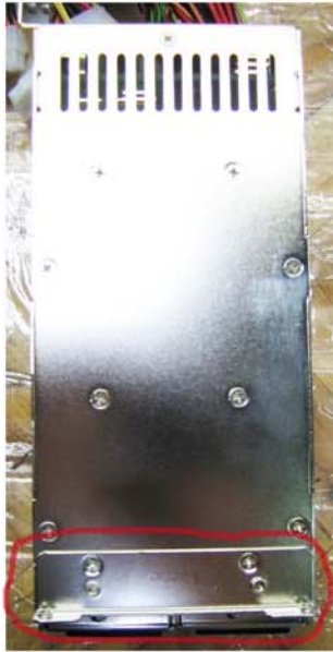
7. Install the PSU into the chassis and fix it with the holes marked in red.
