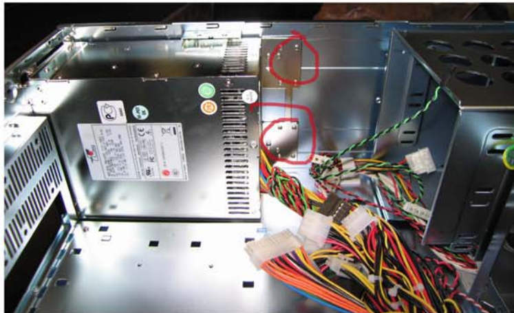
7. Install the PSU into the chassis and fix it with the holes marked in red.
