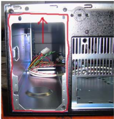
6. Remove the pre-installed ATX bracket from the chassis
