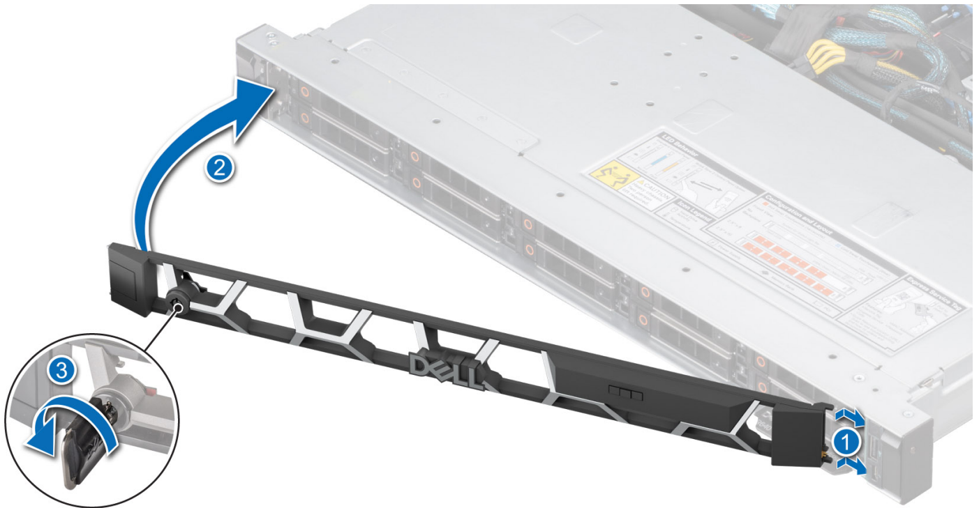
Figure 21. Installing the front bezel with the LCD panel
