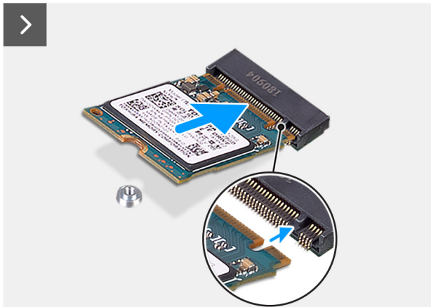
Figure 23. Installing the M.2 2230 PCIe solid state drive
