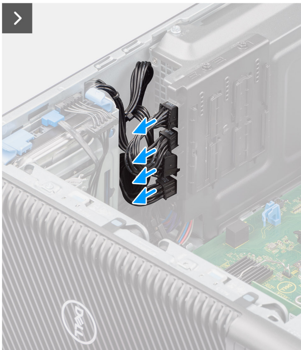
Figure 46. Removing the power-supply unit cover
