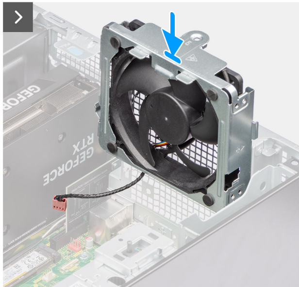
Figure 67. Installing the rear fan (1000W PSU)
