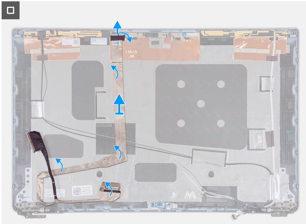
Figure 90. Removing the display cable
