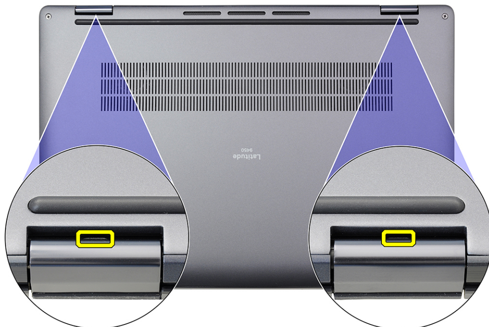
Figure 21. Base cover pry points
