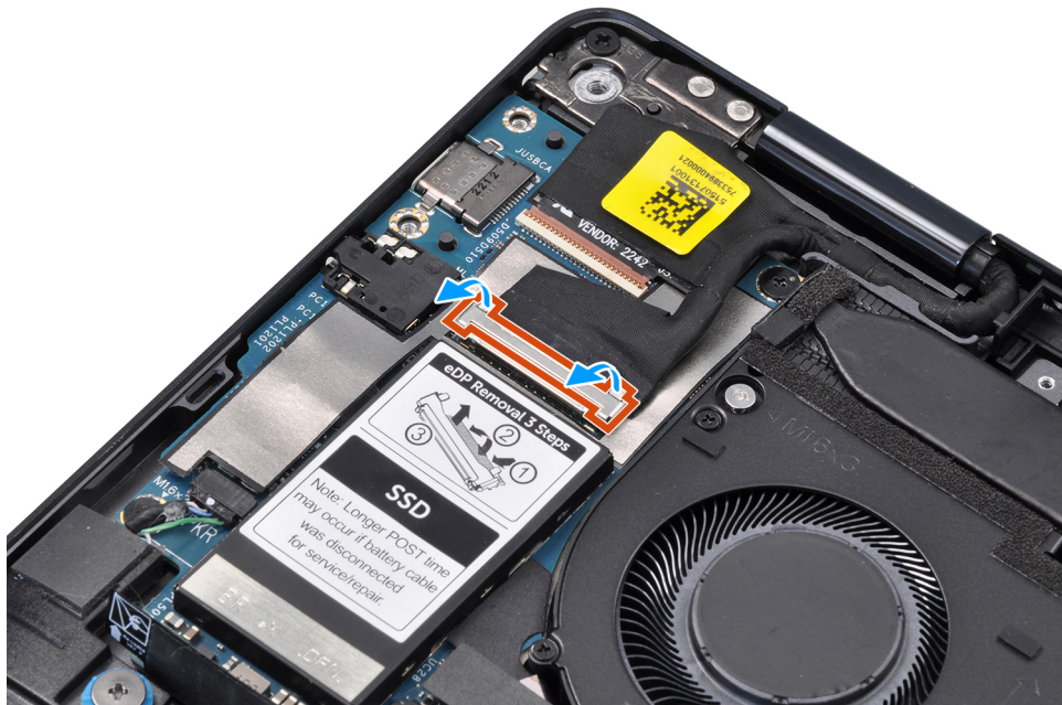
Figure 47. Disconnecting the display cable
