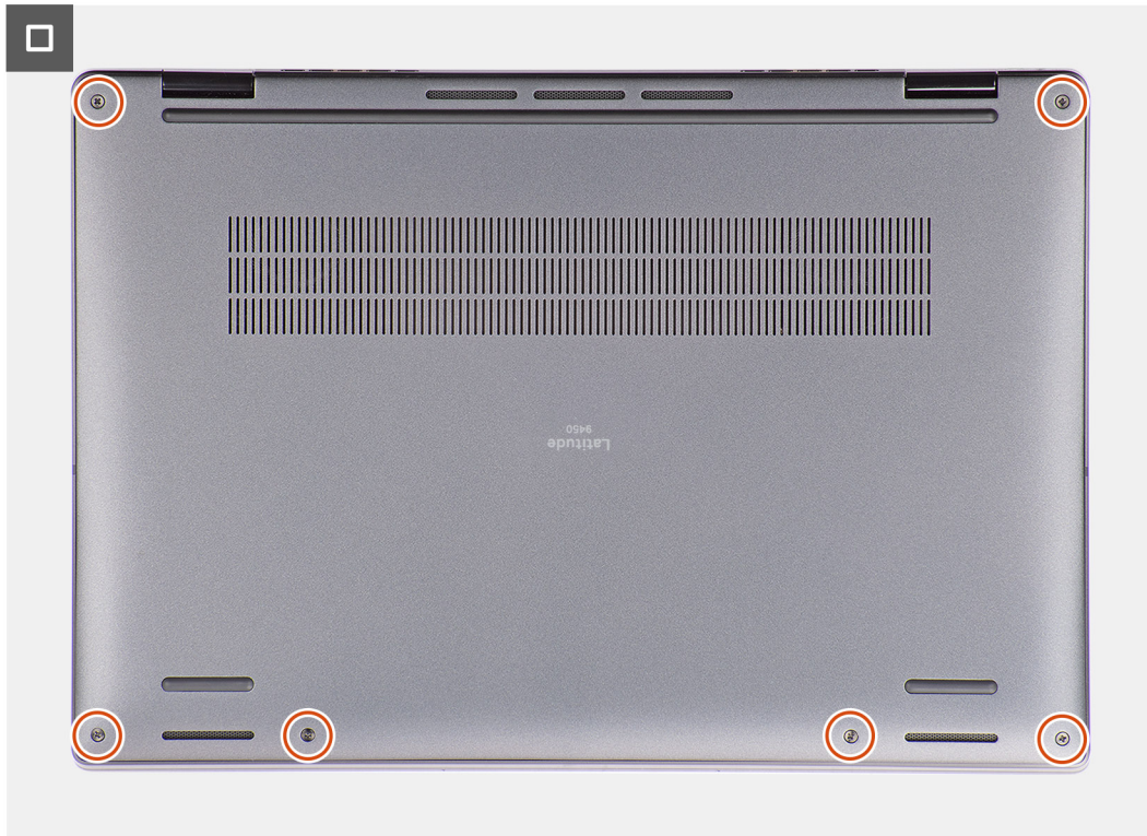
Figure 23. Installing the base cover
