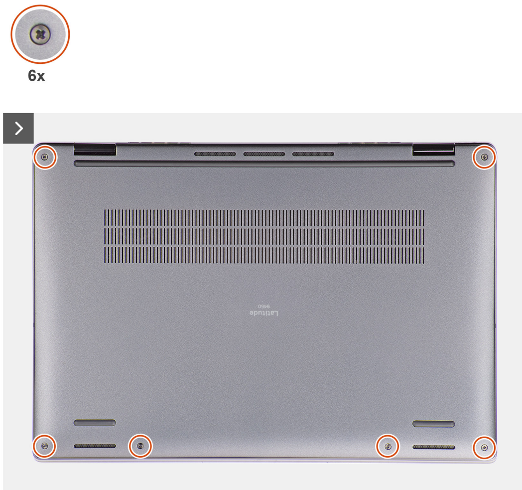
Figure 19. Base cover removal
