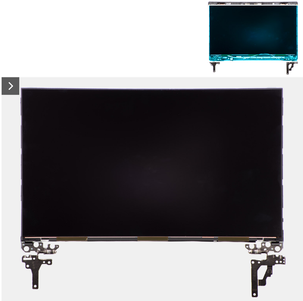
Figure 61. Installing the display panel
