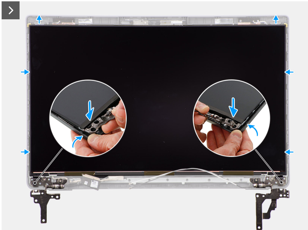
Figure 64. Installing the display panel
