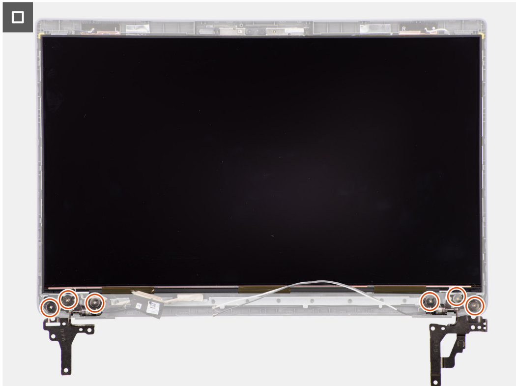
Figure 65. Installing the display panel
