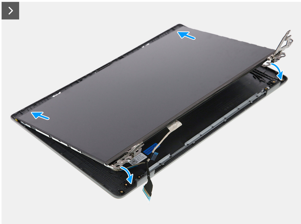
Figure 63. Installing the display panel
