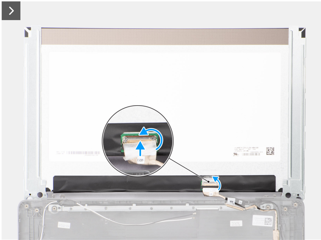
Figure 62. Installing the display panel
