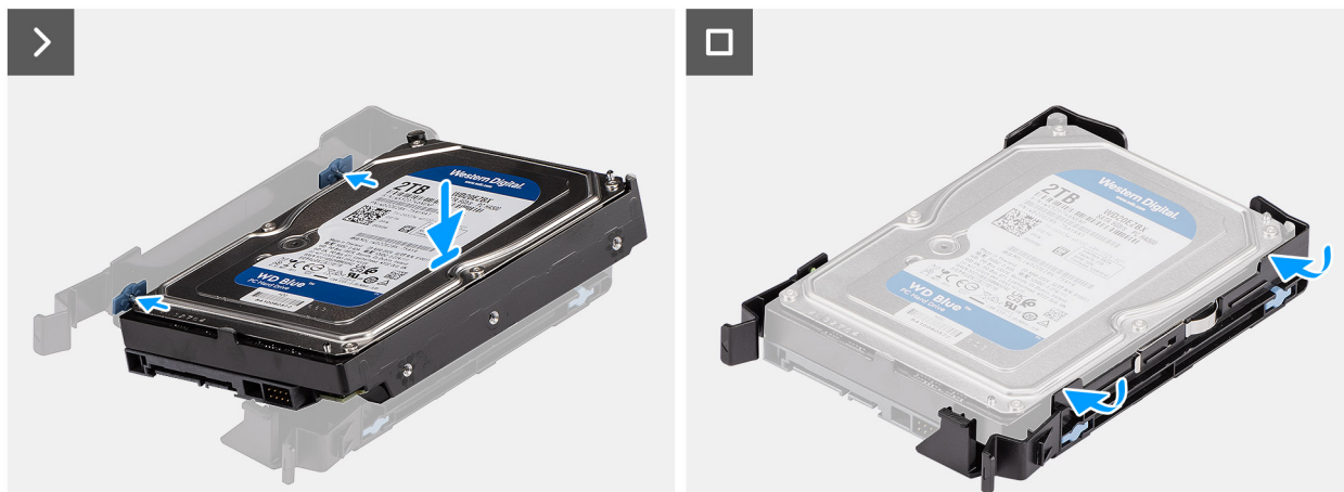
Figure 29. Installing the 3.5-inch hard drive bracket
