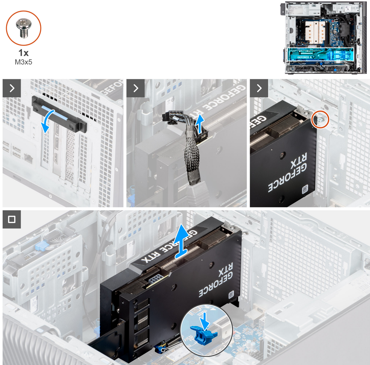
Figure 40. Removing the powered graphics card
