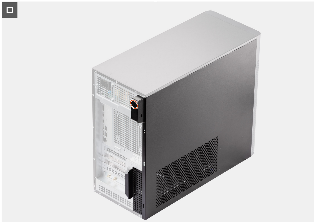
Figure 13. Installing the side cover
