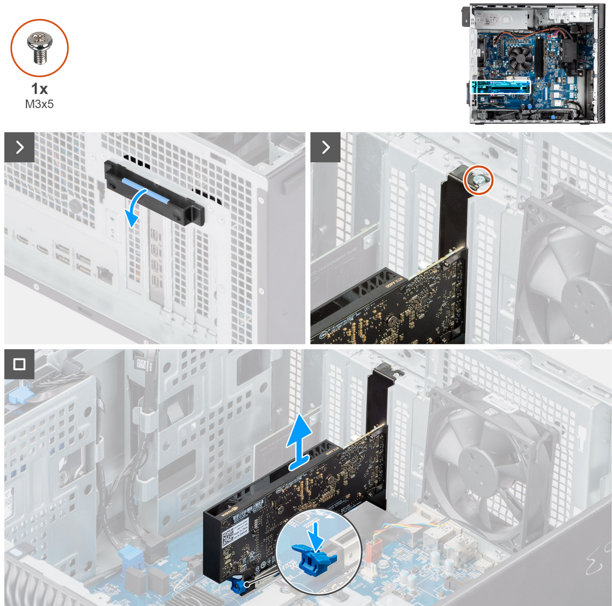
Figure 38. Removing the graphics card
