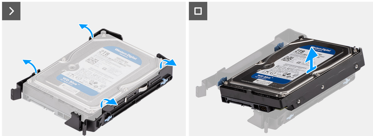
Figure 28. Removing the 3.5-inch hard-disk drive bracket
