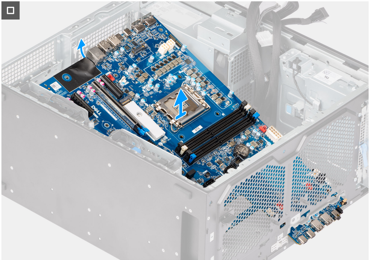
Figure 93. Removing the system board
