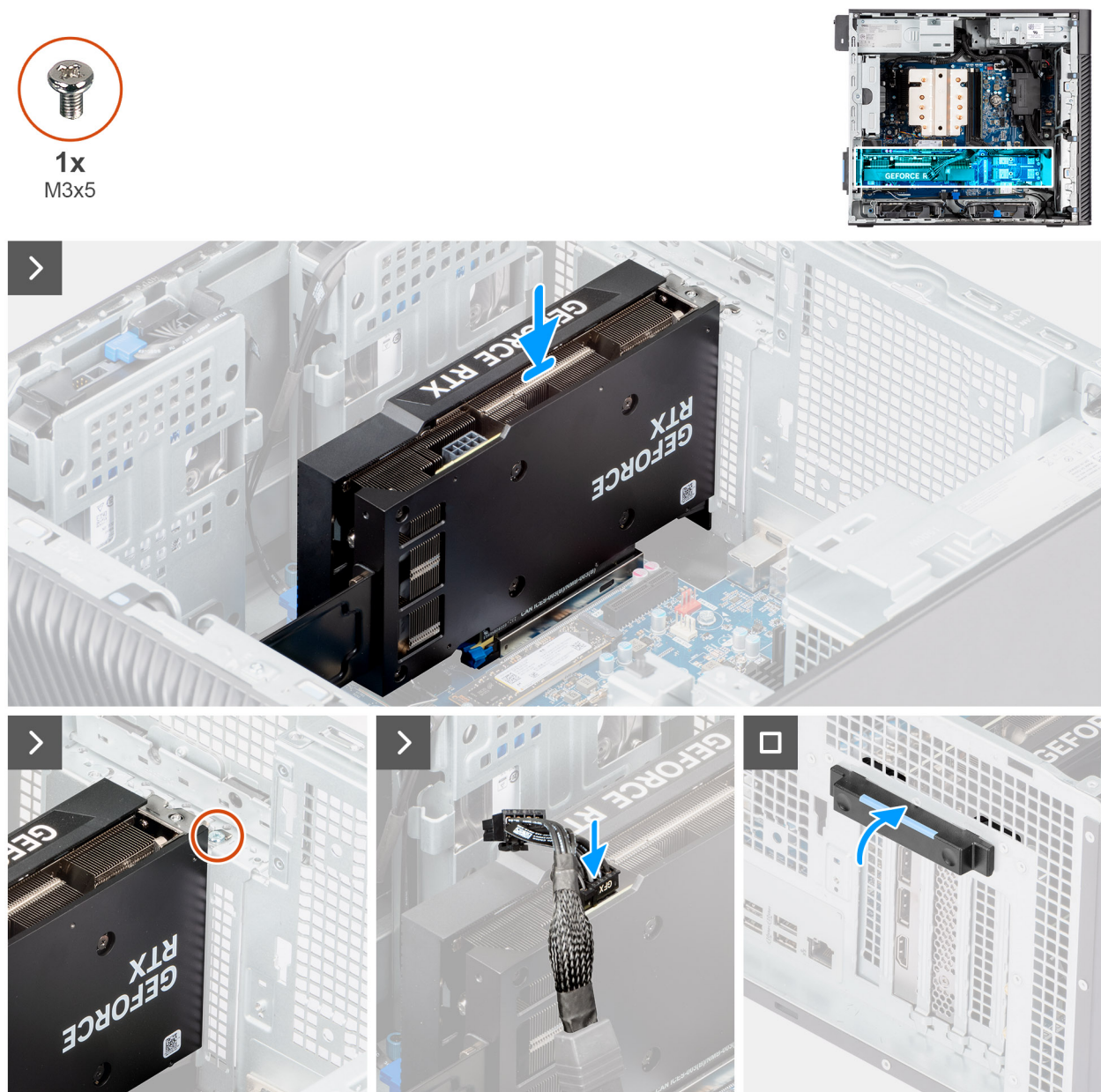
Figure 41. Installing the powered graphics card
