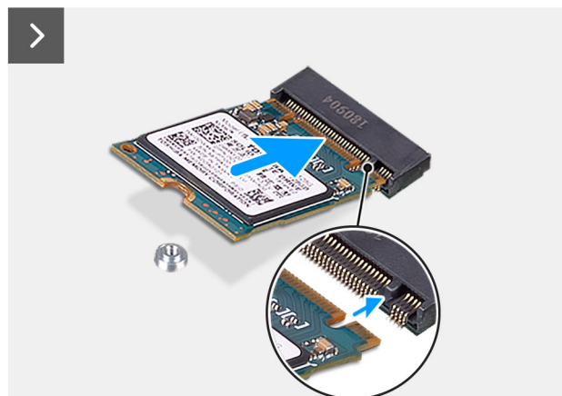
Figure 33. Installing the M.2 2230 PCIe solid state drive
