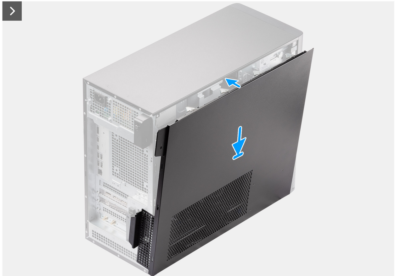
Figure 12. Installing the side cover
