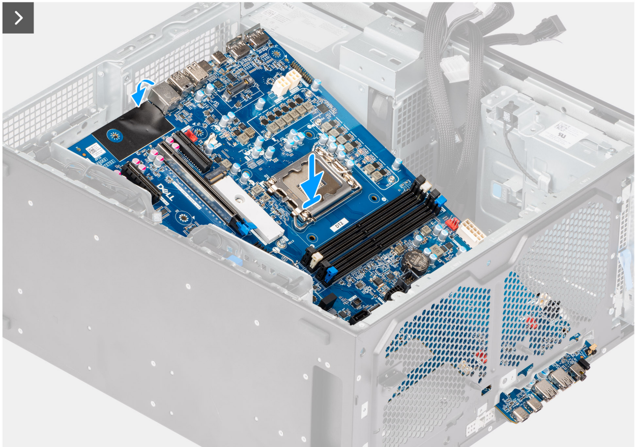
Figure 95. Installing the system board
