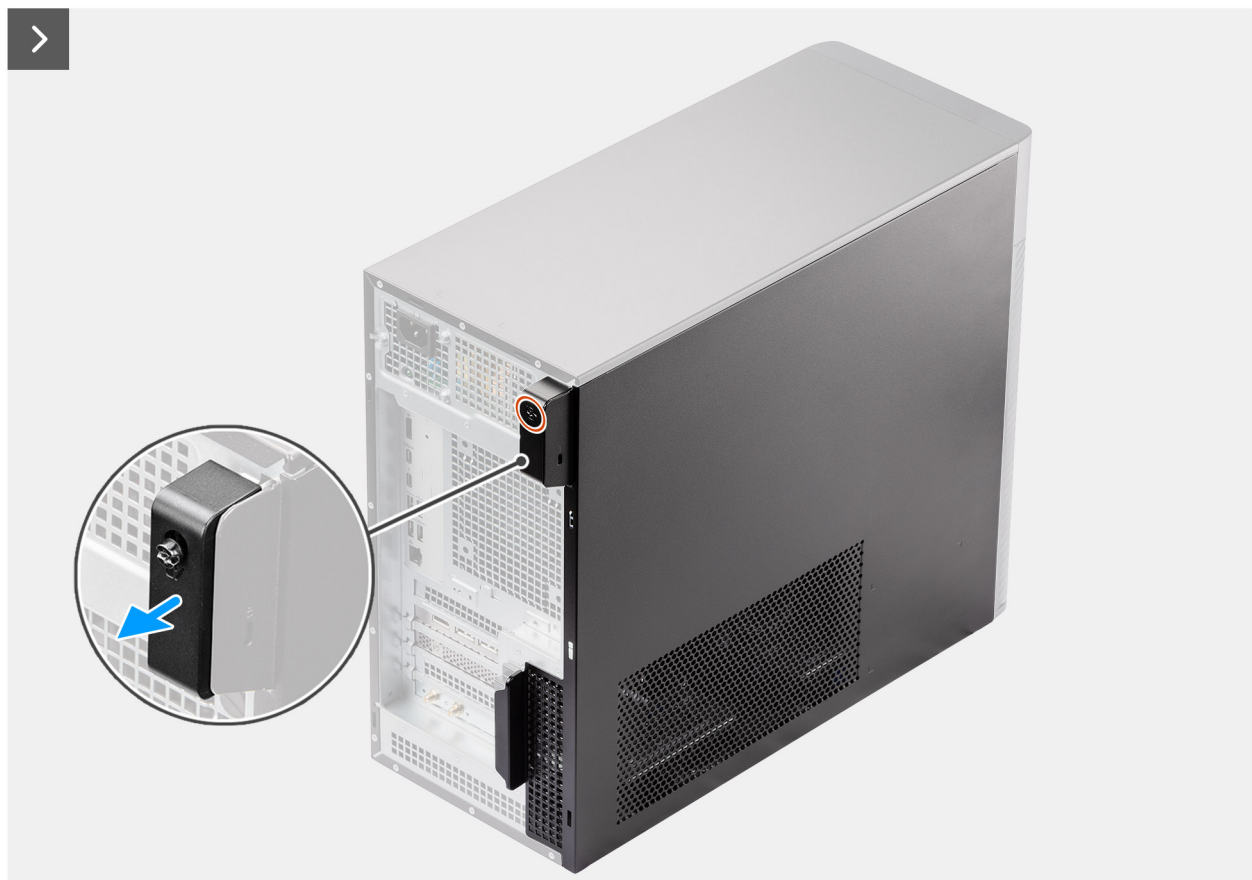
Figure 10. Removing the side cover
