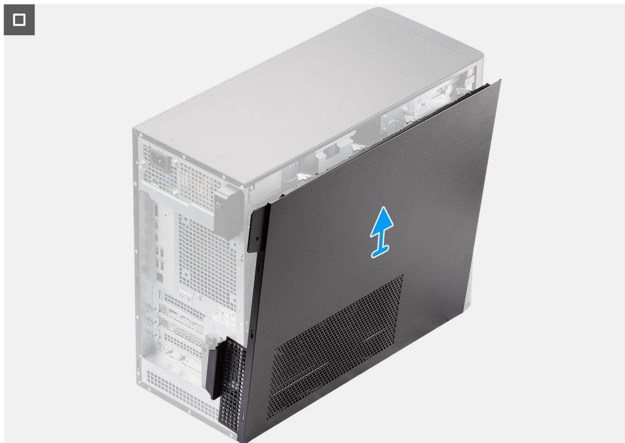
Figure 11. Removing the side cover
