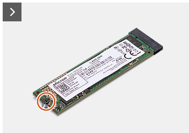
Figure 34. Removing the M.2 2280 PCIe solid state drive
