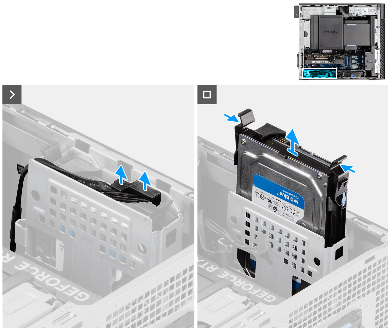
Figure 27. Removing the 3.5-inch hard drive assembly (Bay-2)
