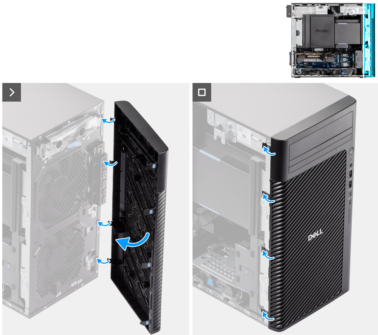
Figure 19. Installing the front bezel
