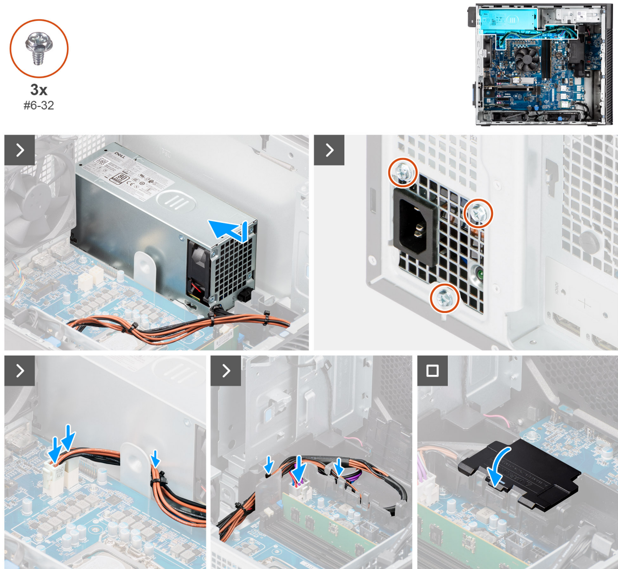
Figure 59. Installing the 360 W power-supply unit
