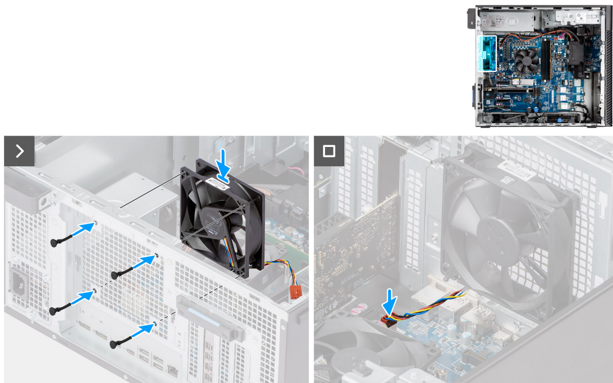
Figure 51. Installing the rear fan for 360 W PSU computers
