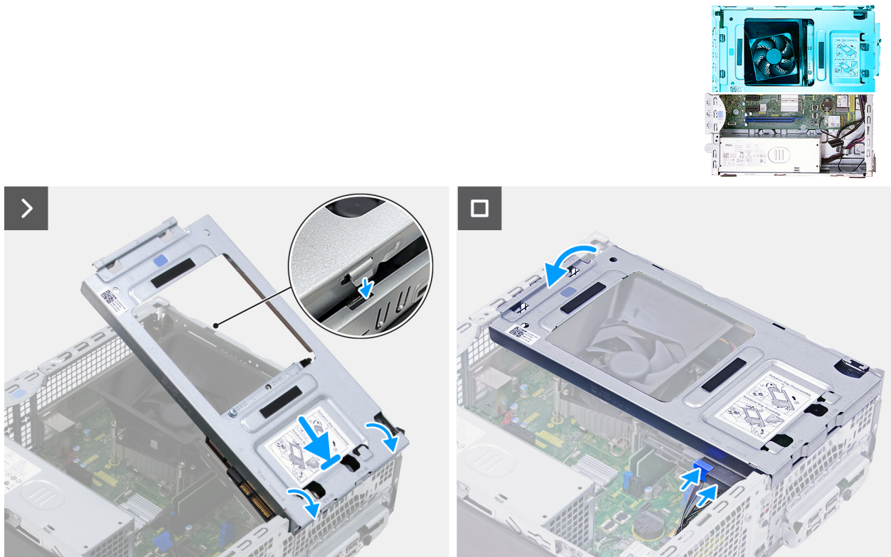
Figure 21. Installing the drive bay
