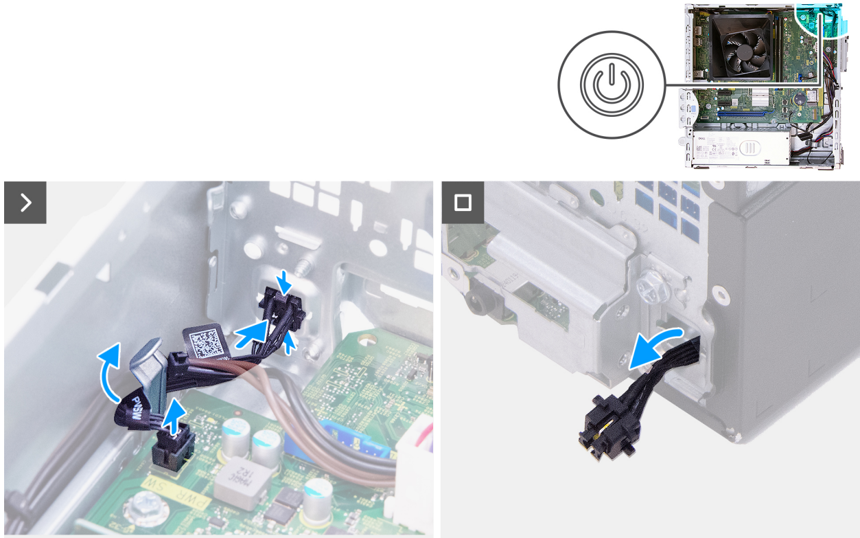
Figure 44. Removing the power button
