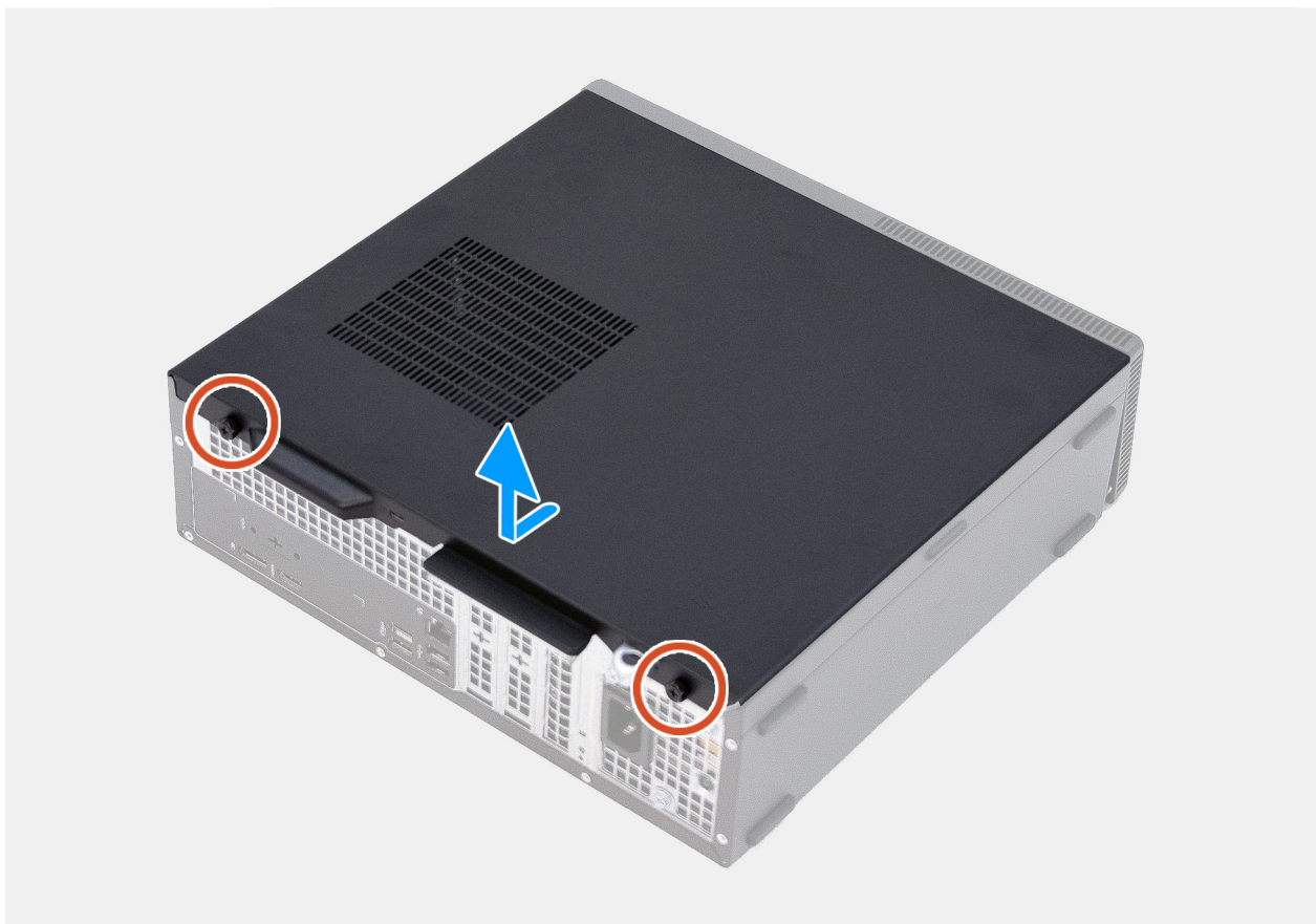
Figure 11. Removing the left-side cover
