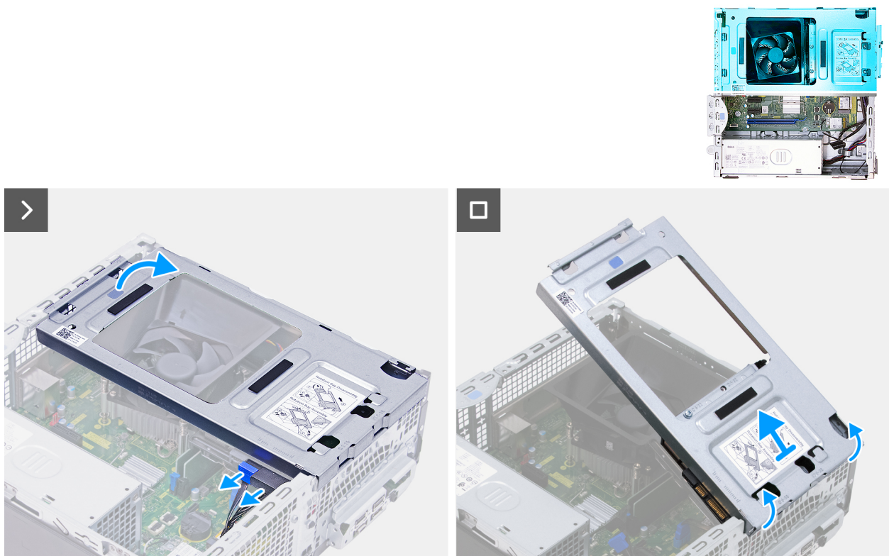
Figure 19. Removing the drive bay
