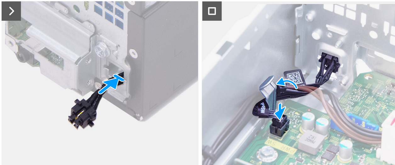
Figure 45. Installing the power button
