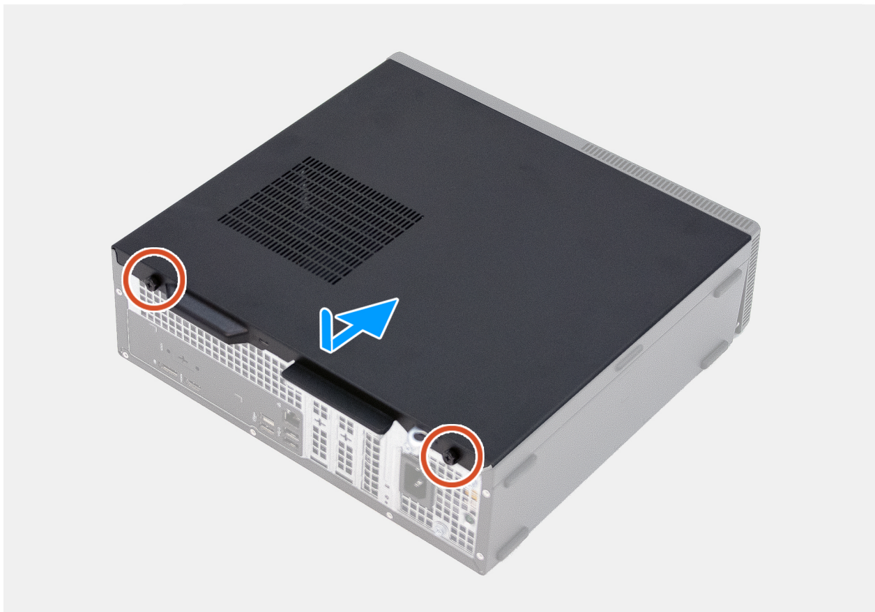
Figure 12. Installing the left-side cover
