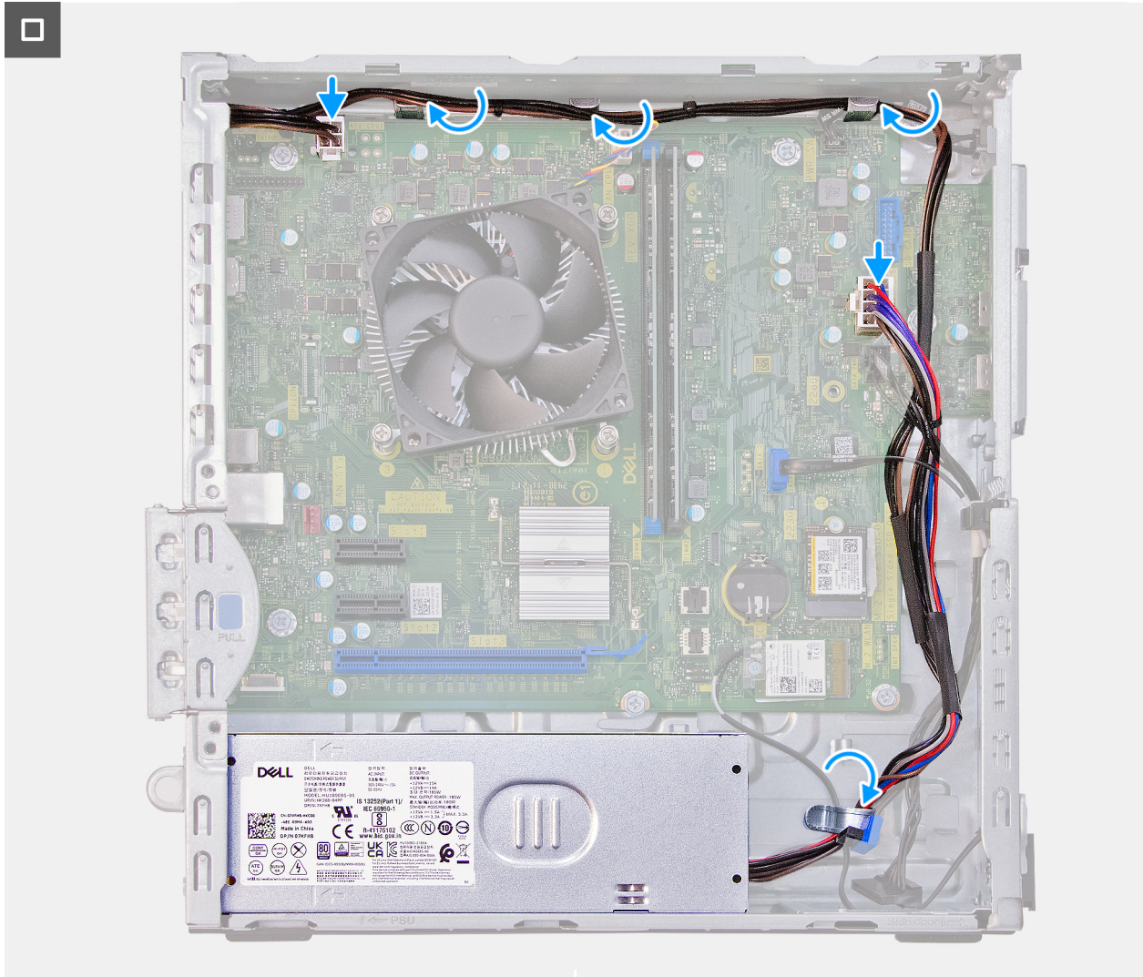
Figure 37. Installing the power-supply unit
