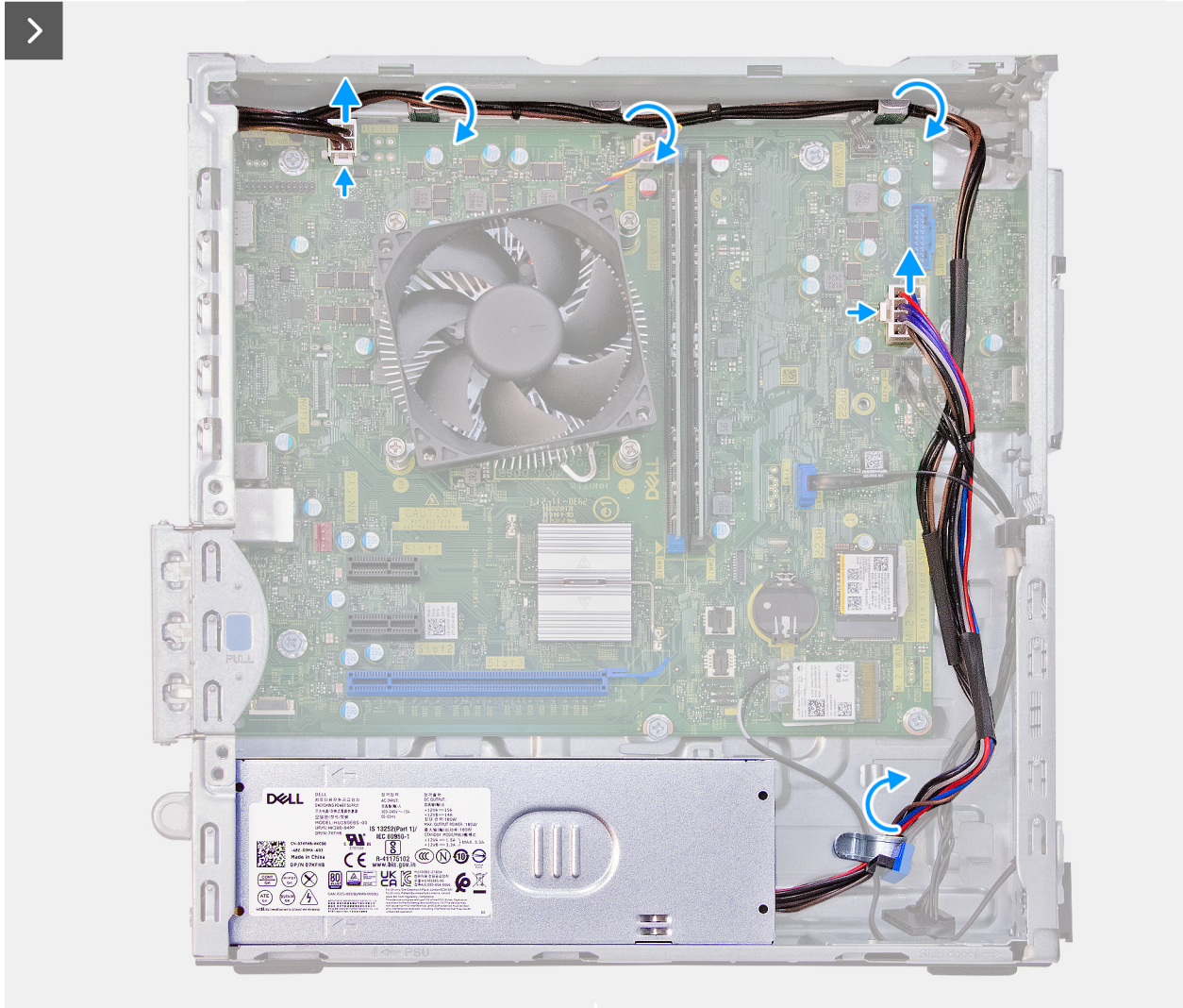
Figure 34. Removing the power-supply unit
