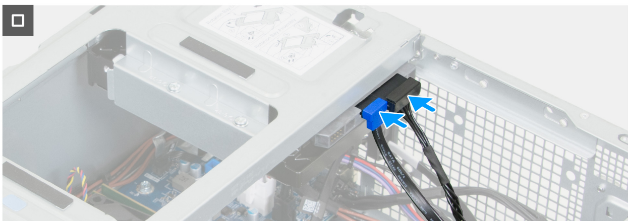
Figure 32. Installing the drive bay
