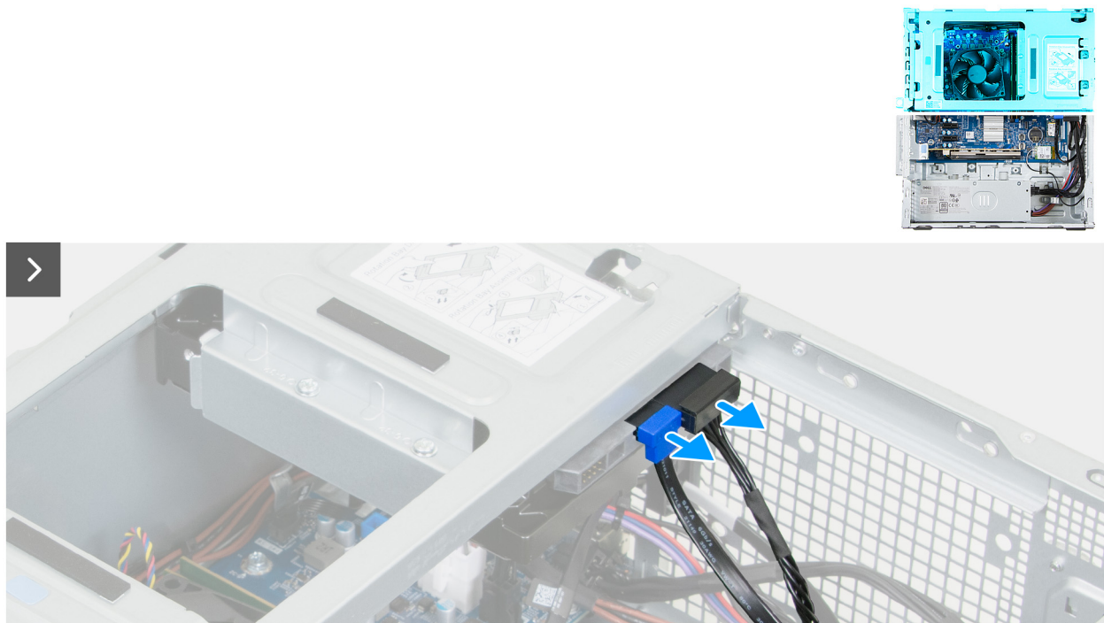
Figure 28. Removing the drive bay
