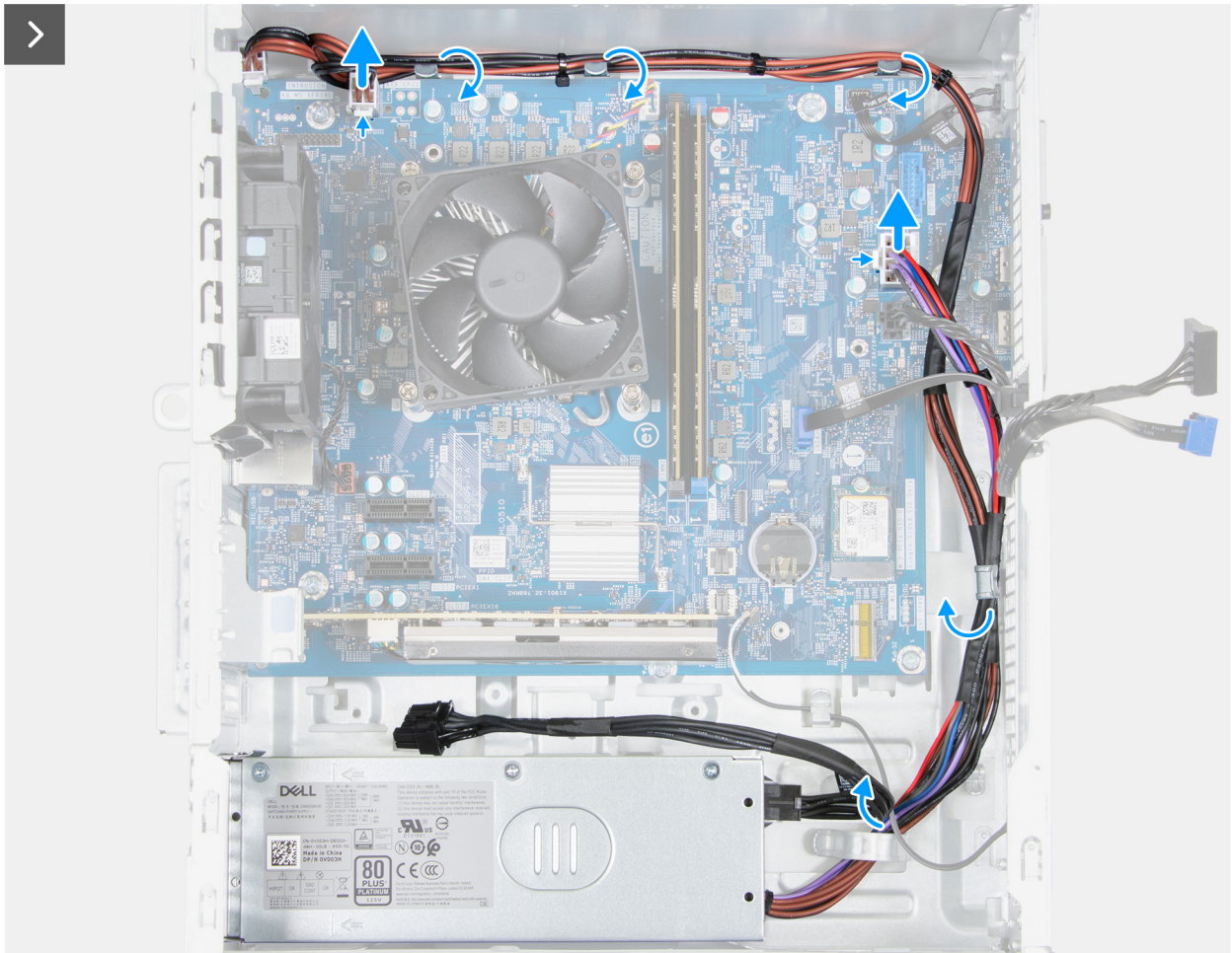
Figure 46. Removing the power-supply unit
