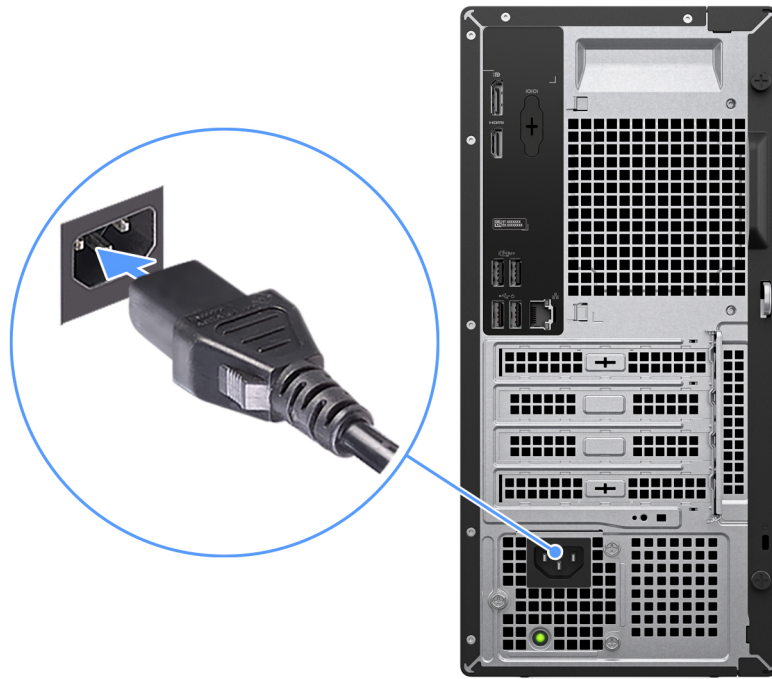
Figure 7. Connecting the power cable
