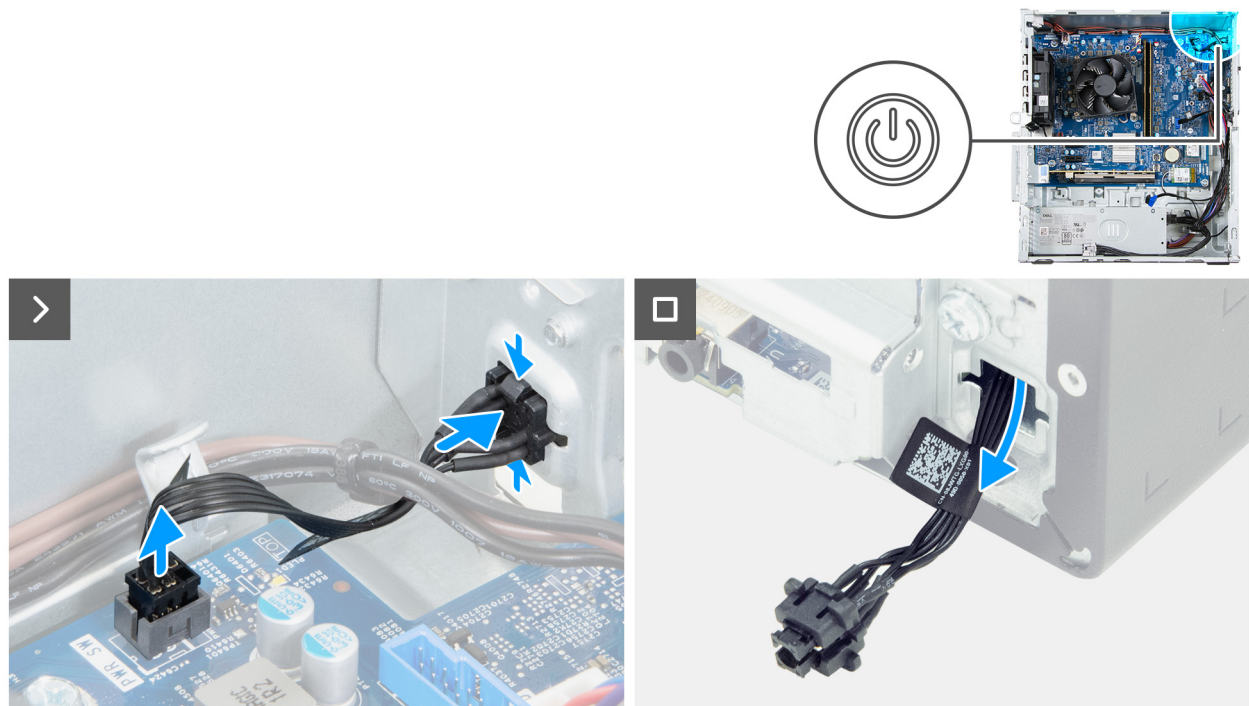
Figure 35. Removing the power button
