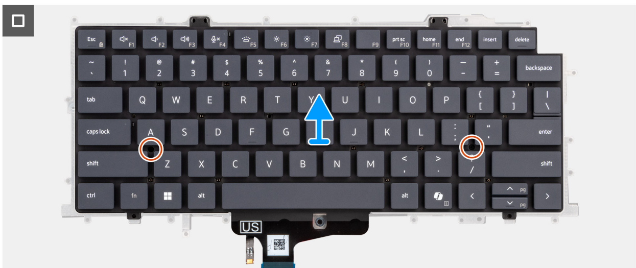
Figure 80. Removing the keyboard
