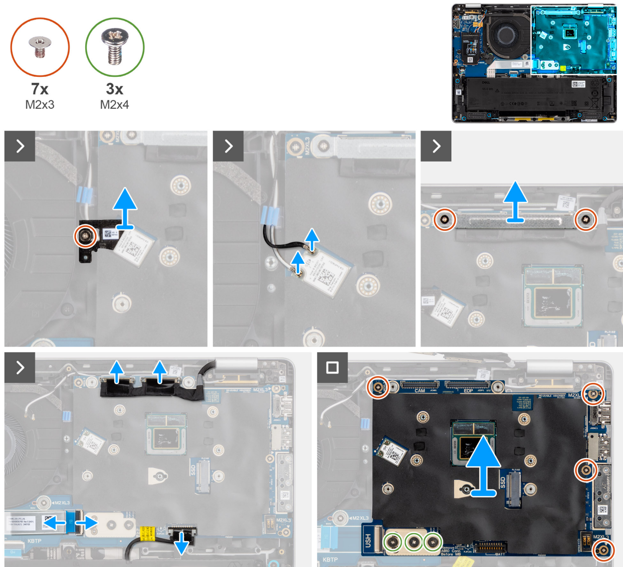
Figure 70. Removing the system board
