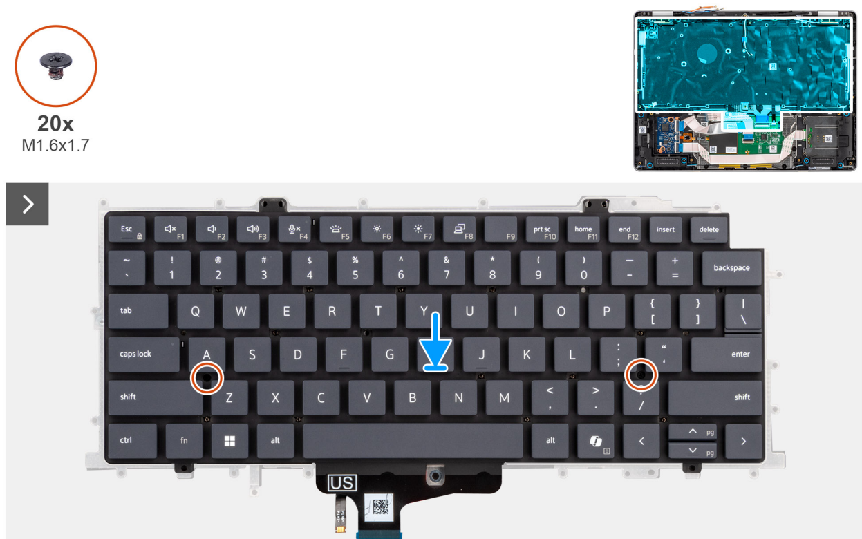
Figure 81. Installing the keyboard
