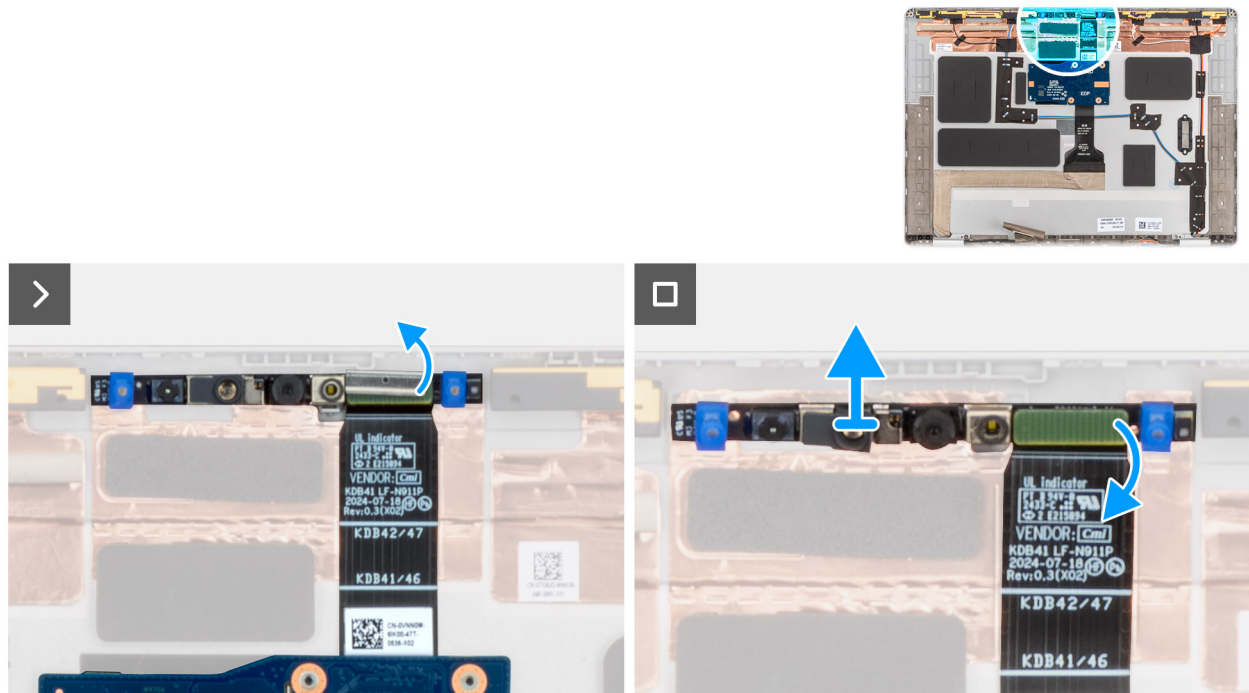
Figure 56. Removing the MIPI camera
