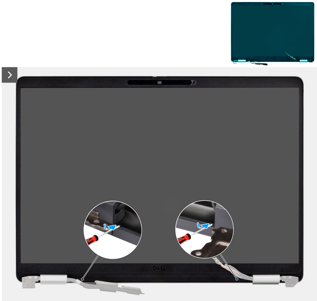
Figure 43. Prying the plastic bezel
