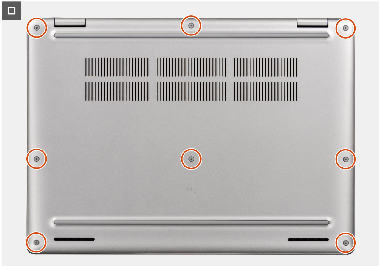
Figure 23. Installing the base cover
