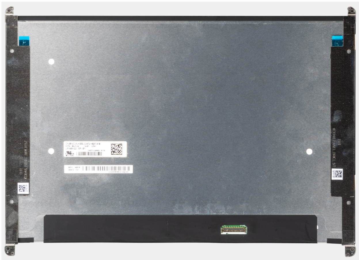
Figure 51. Display panel with brackets
