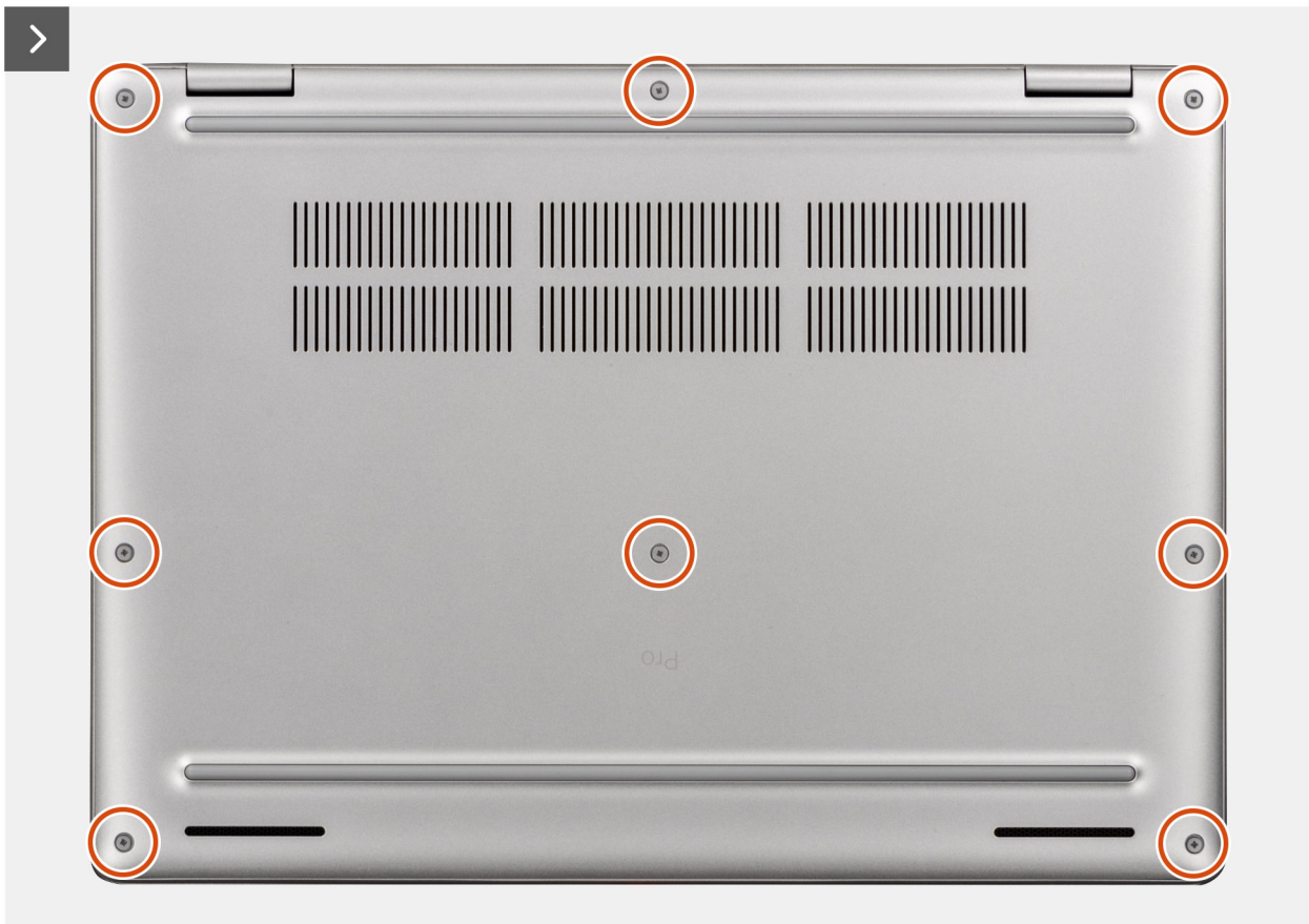
Figure 19. Removing the base cover
