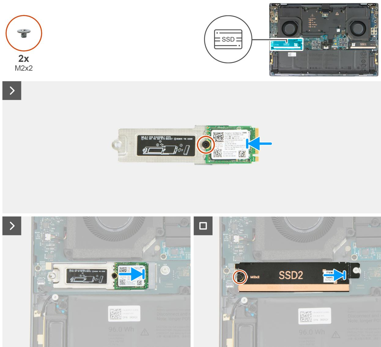
**Figure 29. Installing the M.2 2230 solid state drive (SSD2)**
