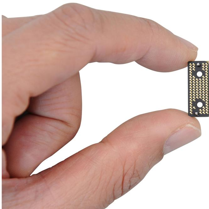
**Figure 45. Handling of the display-assembly cable interposer board**
