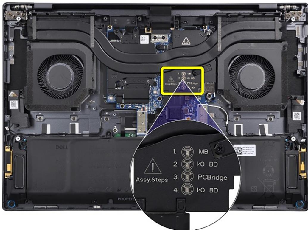
**Figure 57. Assembly steps printed on the heat sink**
