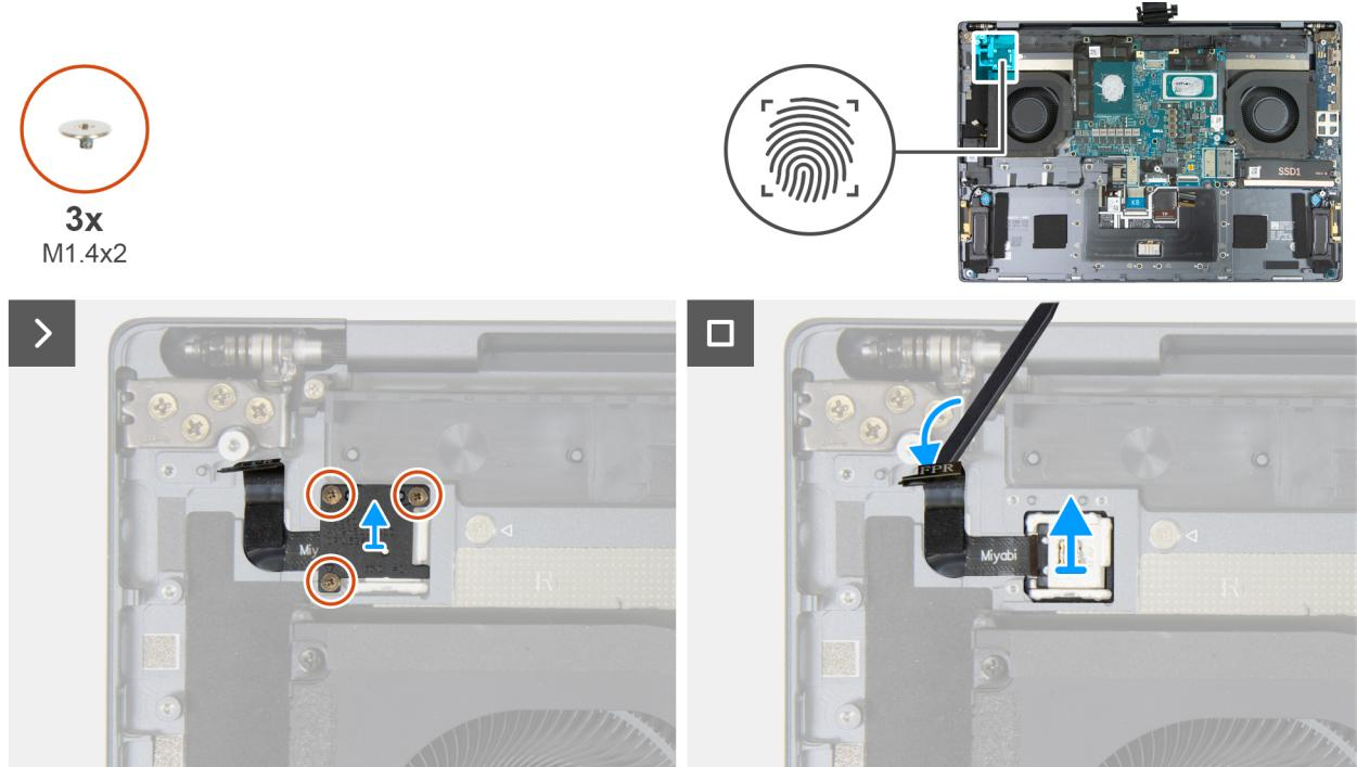
**Figure 72. Removing the power button or fingerprint reader**
