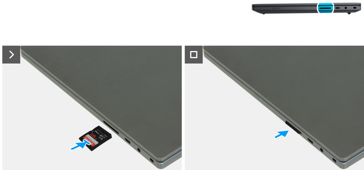
**Figure 12. Installing the memory card**
