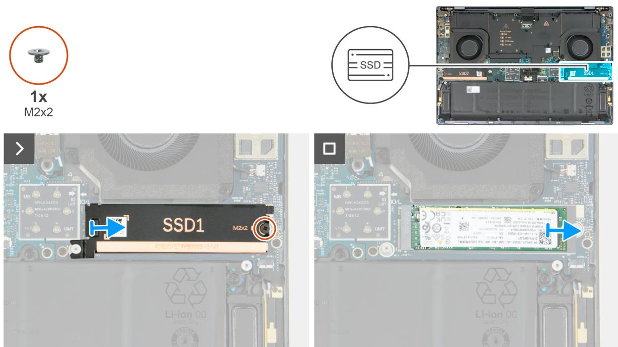
**Figure 22. Removing the M.2 2280 solid state drive (SSD1)**
