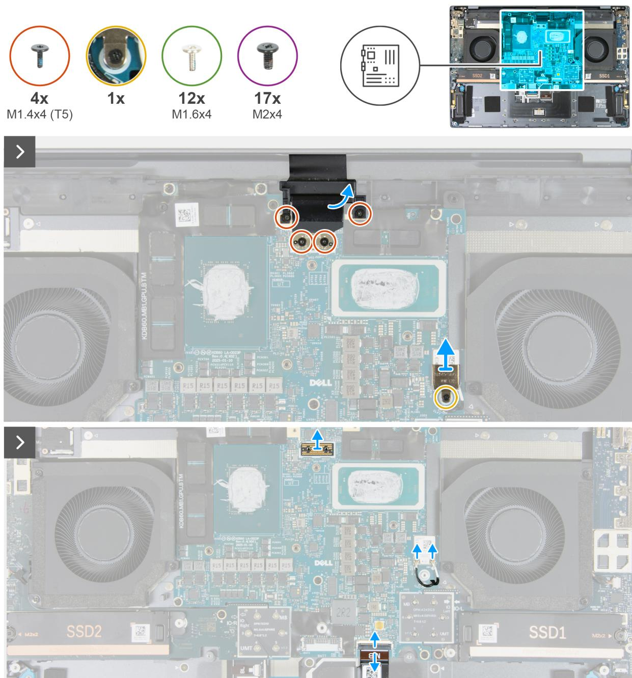
**Figure 64. Removing the system board (discrete graphics)**
