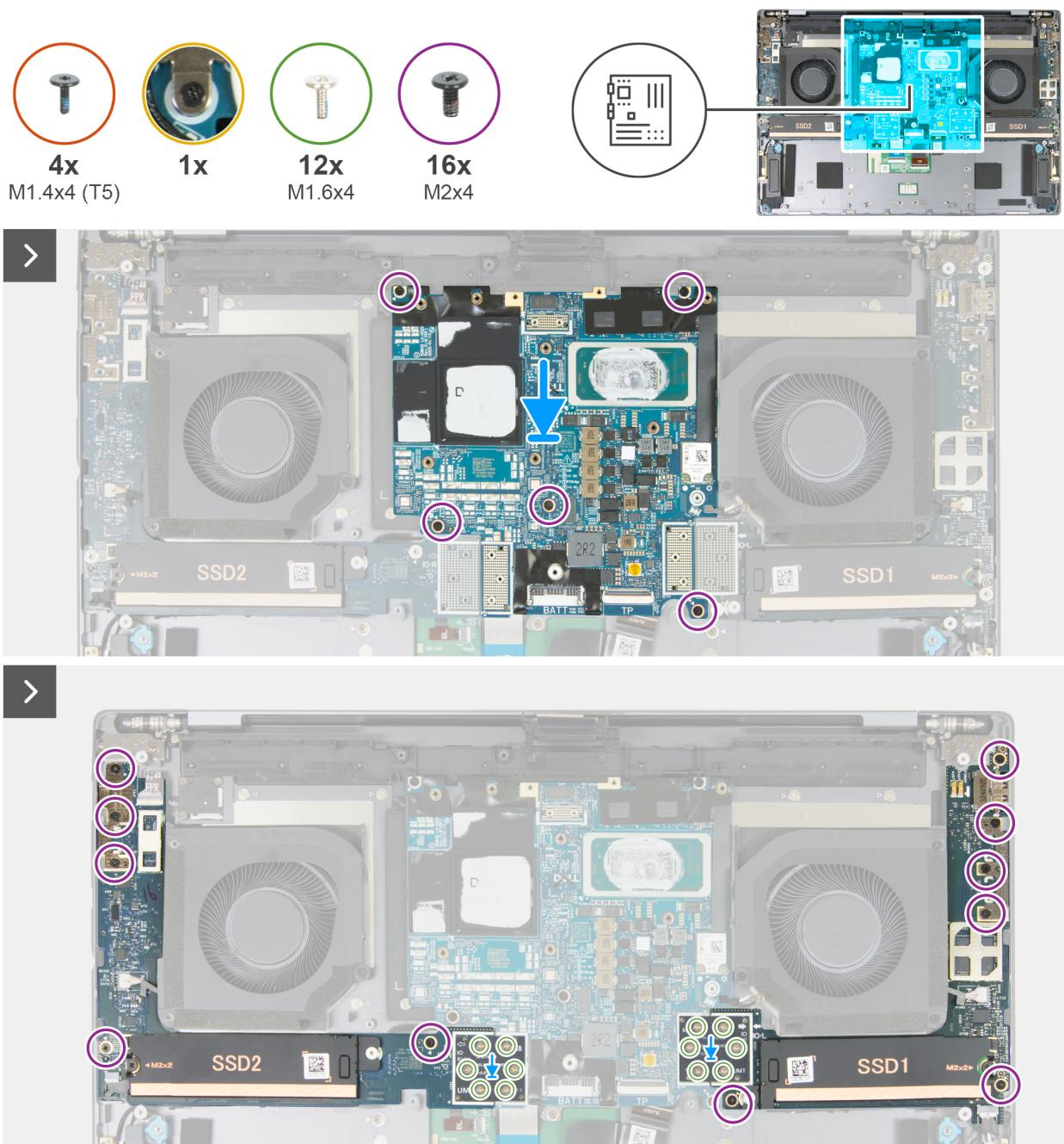
**Figure 59. Installing the system board (integrated graphics)**
