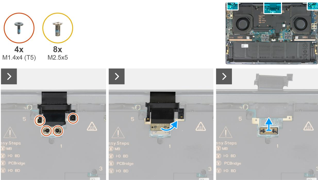
**Figure 34. Removing the display assembly**
