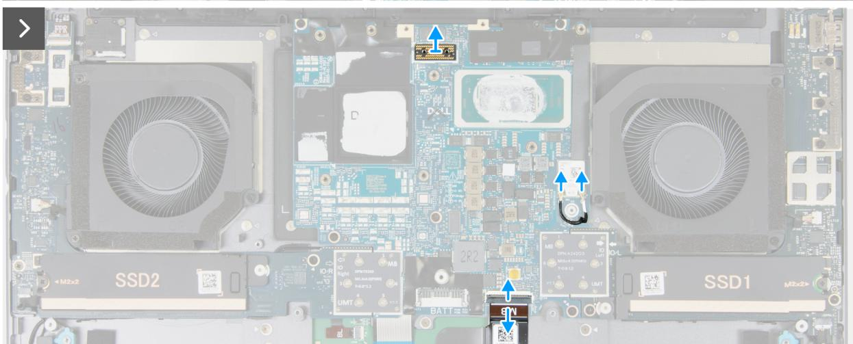
**Figure 55. Removing the system board (integrated graphics)**
