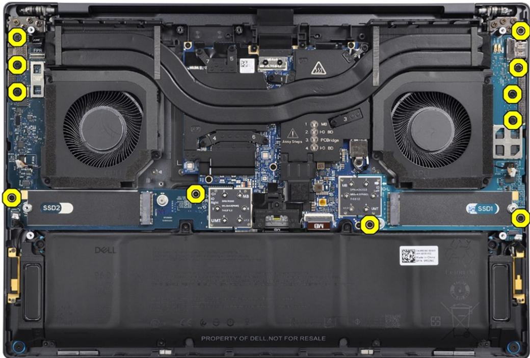
**Figure 70. Screws of I/O boards**
