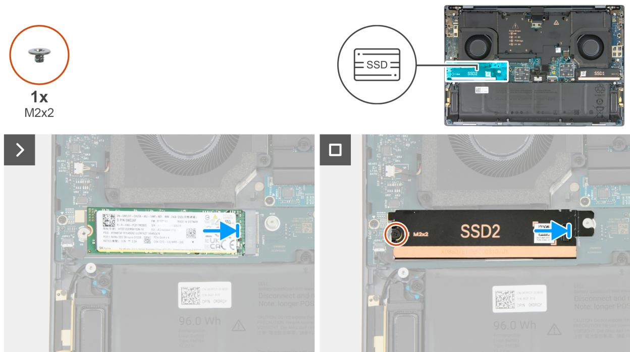
**Figure 25. Installing the M.2 2280 solid state drive (SSD2)**
