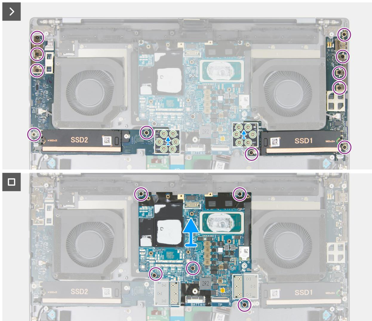
**Figure 56. Removing the system board (integrated graphics)**
