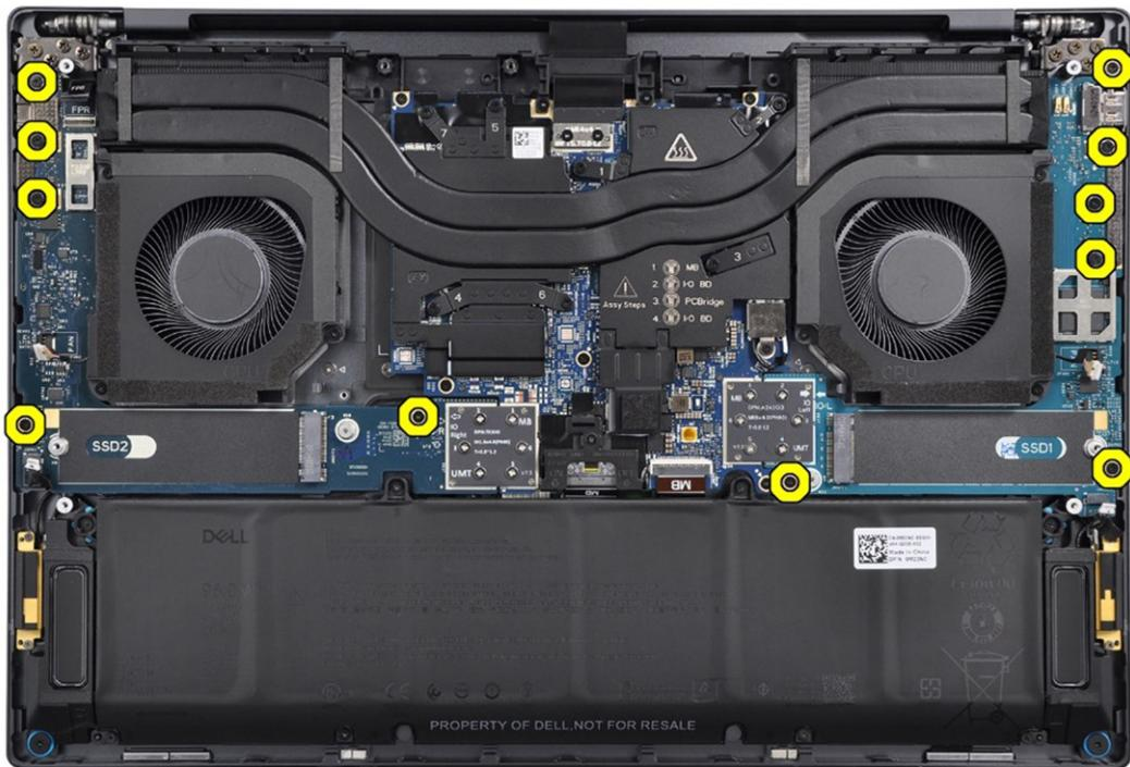
**Figure 61. Screws of I/O boards**
