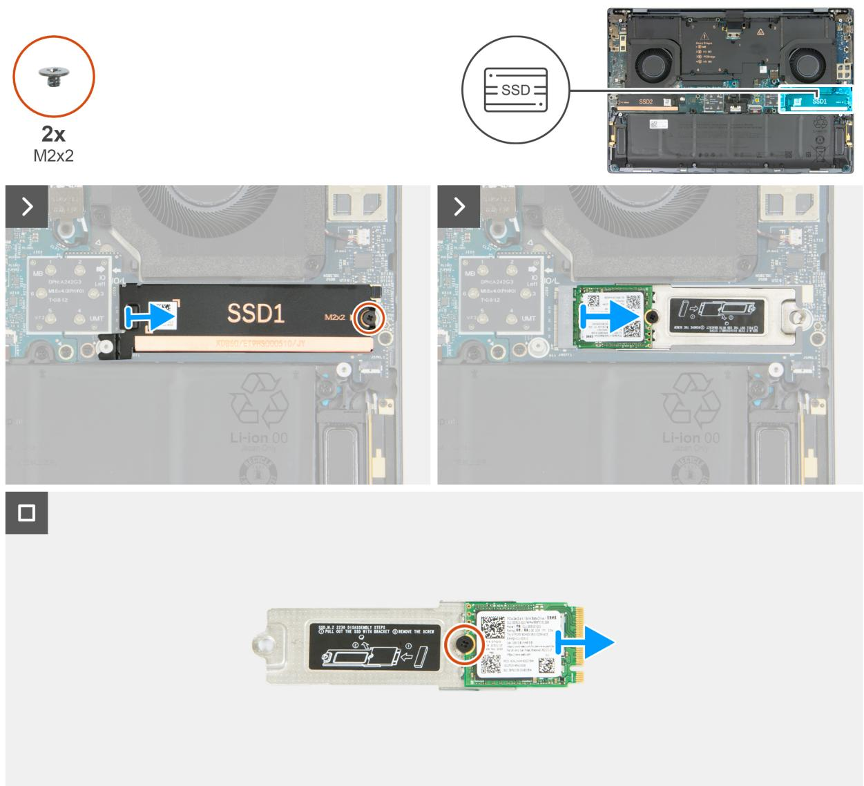
Figure 26. Removing the M.2 2230 solid state drive (SSD1)
