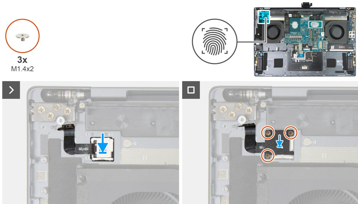
**Figure 73. Installing the power button or fingerprint reader**
