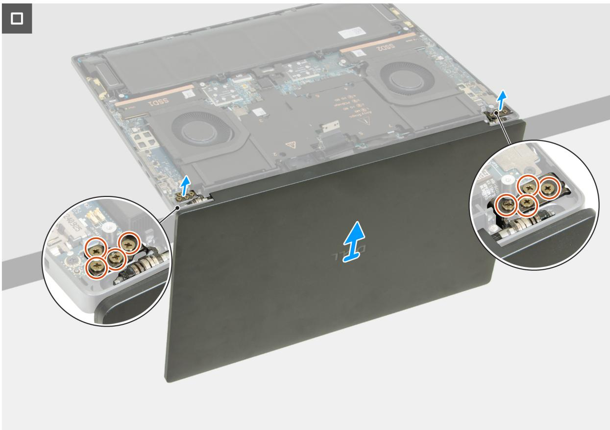
**Figure 35. Removing the display assembly**
