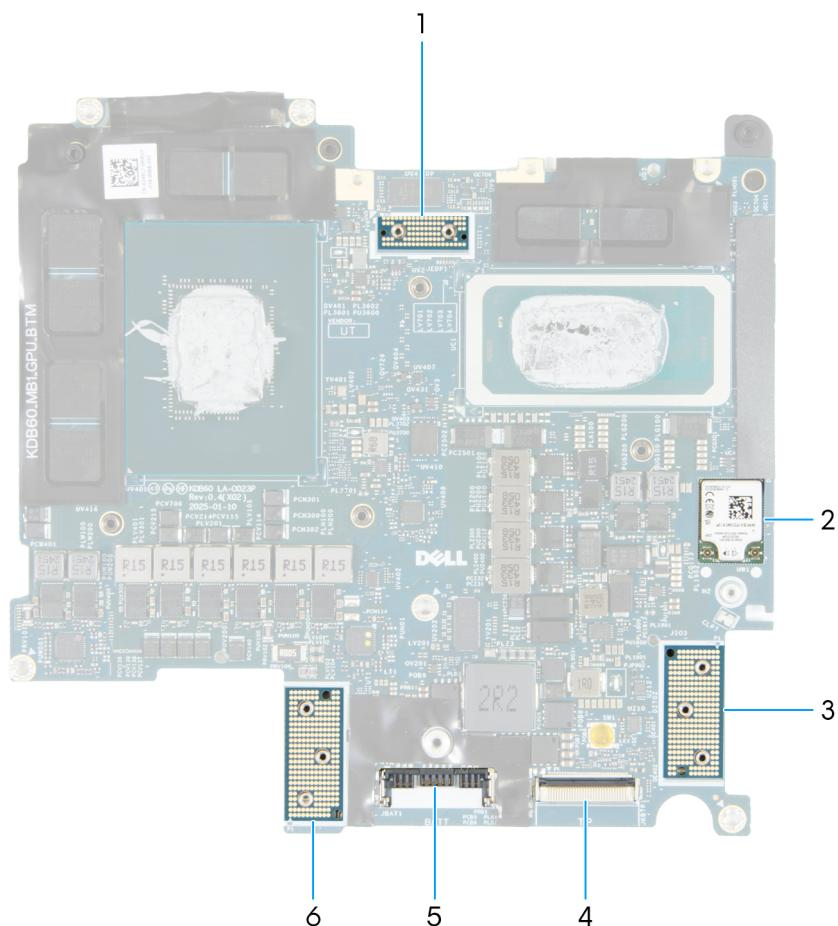
**Figure 63. System board connectors**
