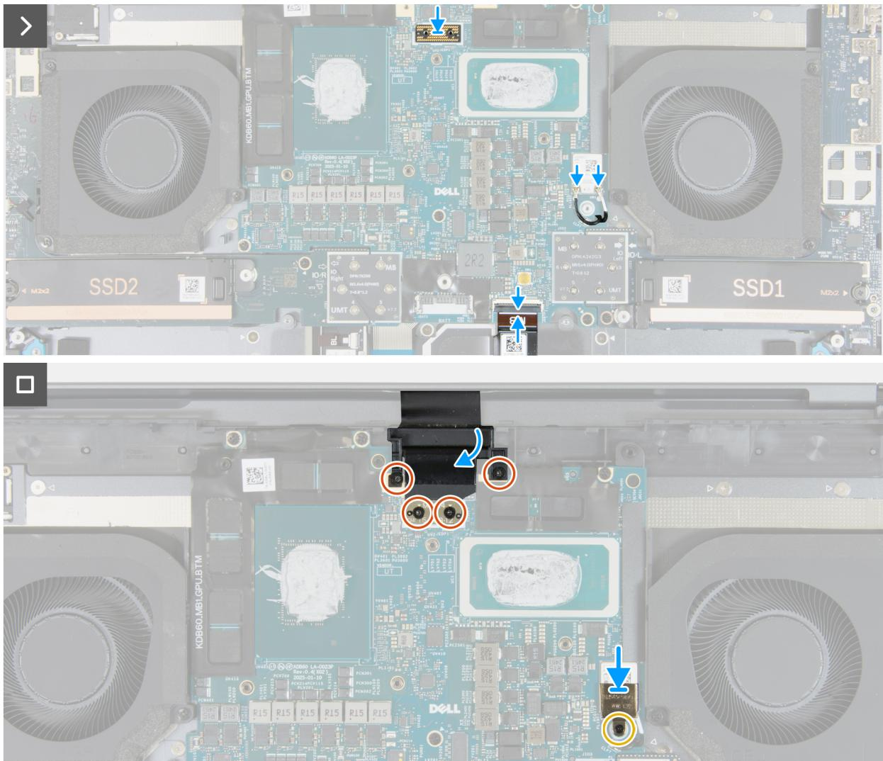
**Figure 69. Installing the system board (discrete graphics)**
