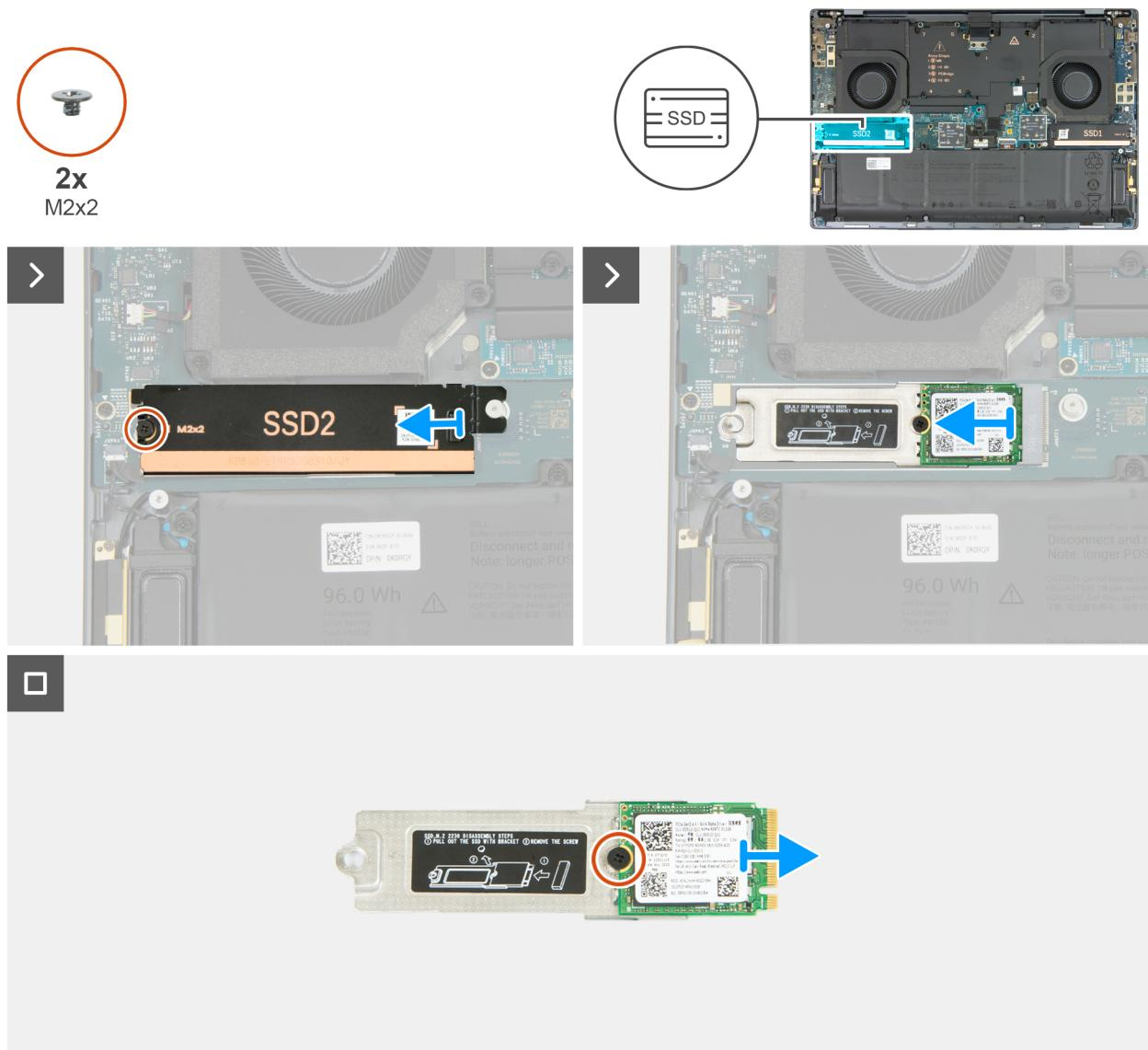
**Figure 27. Removing the M.2 2230 solid state drive (SSD2)**
