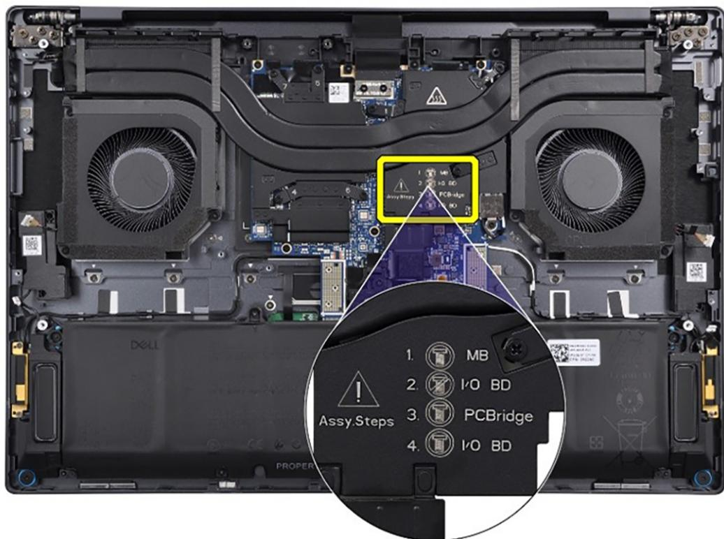
**Figure 62. Assembly steps printed on heat sink**
