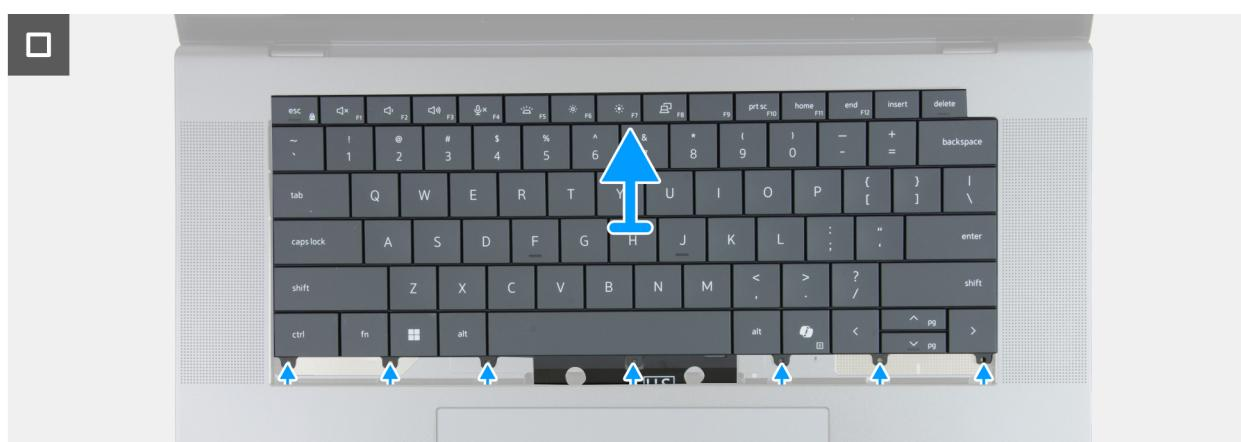
**Figure 77. Removing the keyboard**
