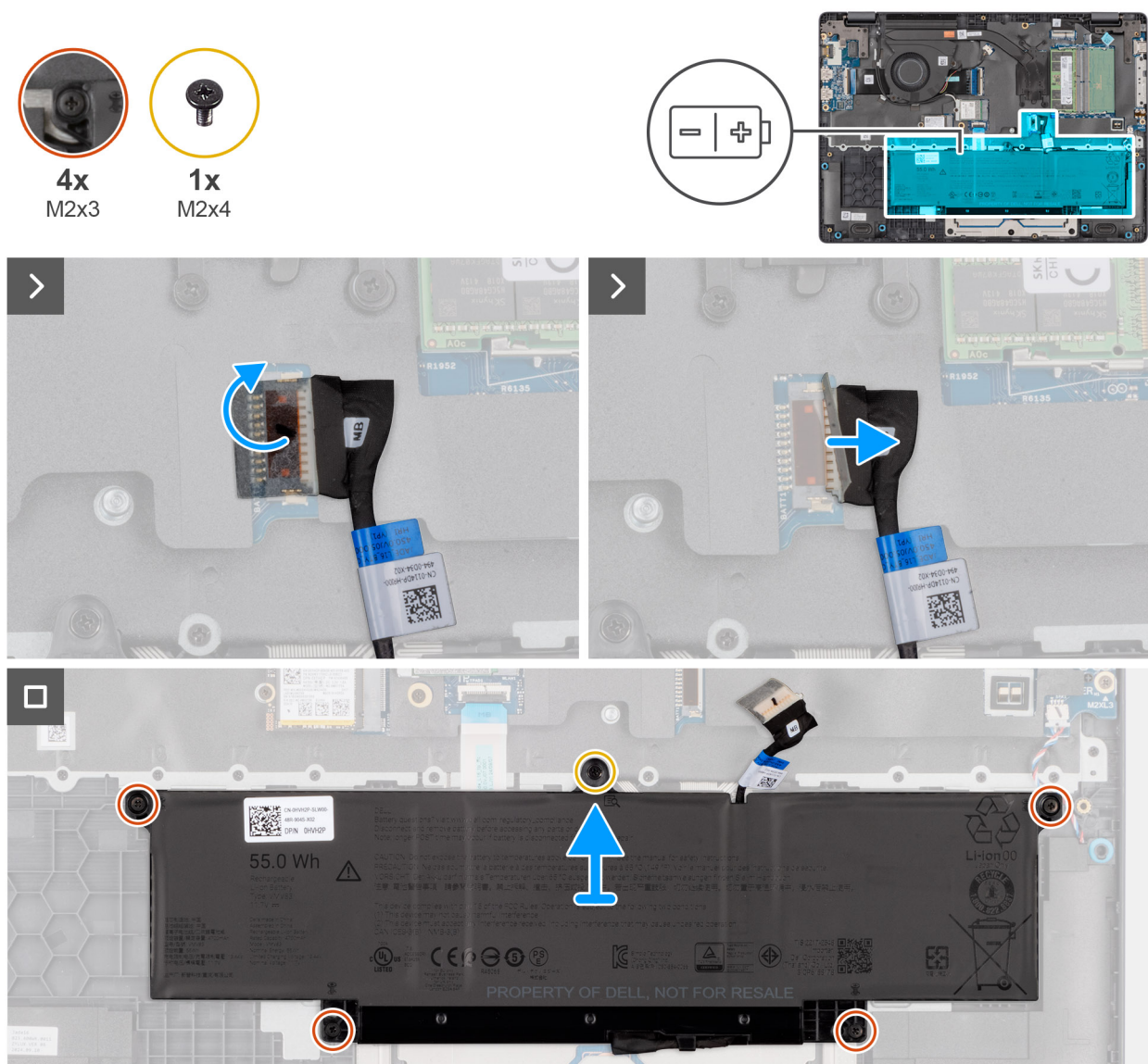
Figure 17. Removing the battery
