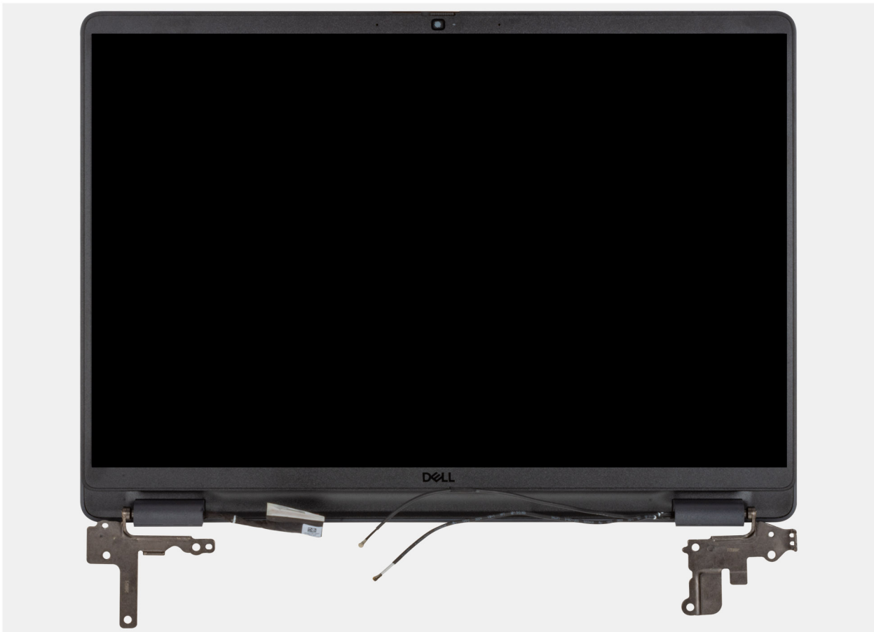
Figure 64. Removing the display assembly
