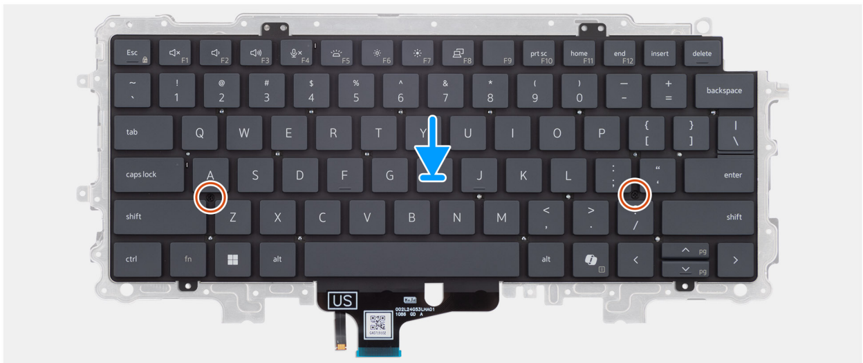
Figure 59. Installing the keyboard support plate
