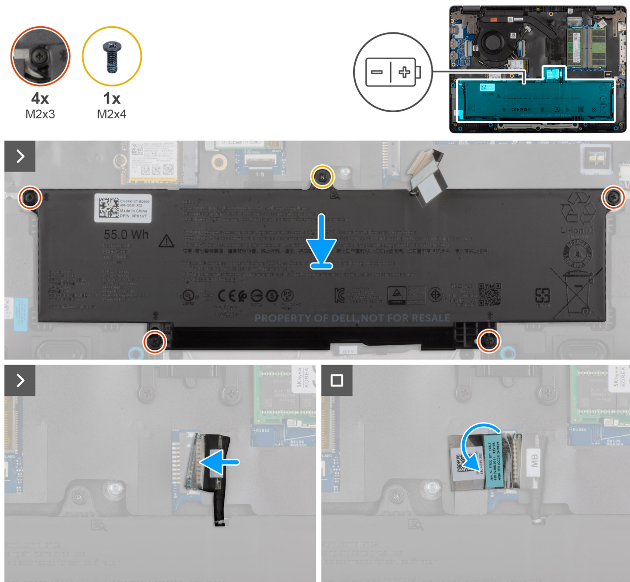
Figure 18. Installing the battery
