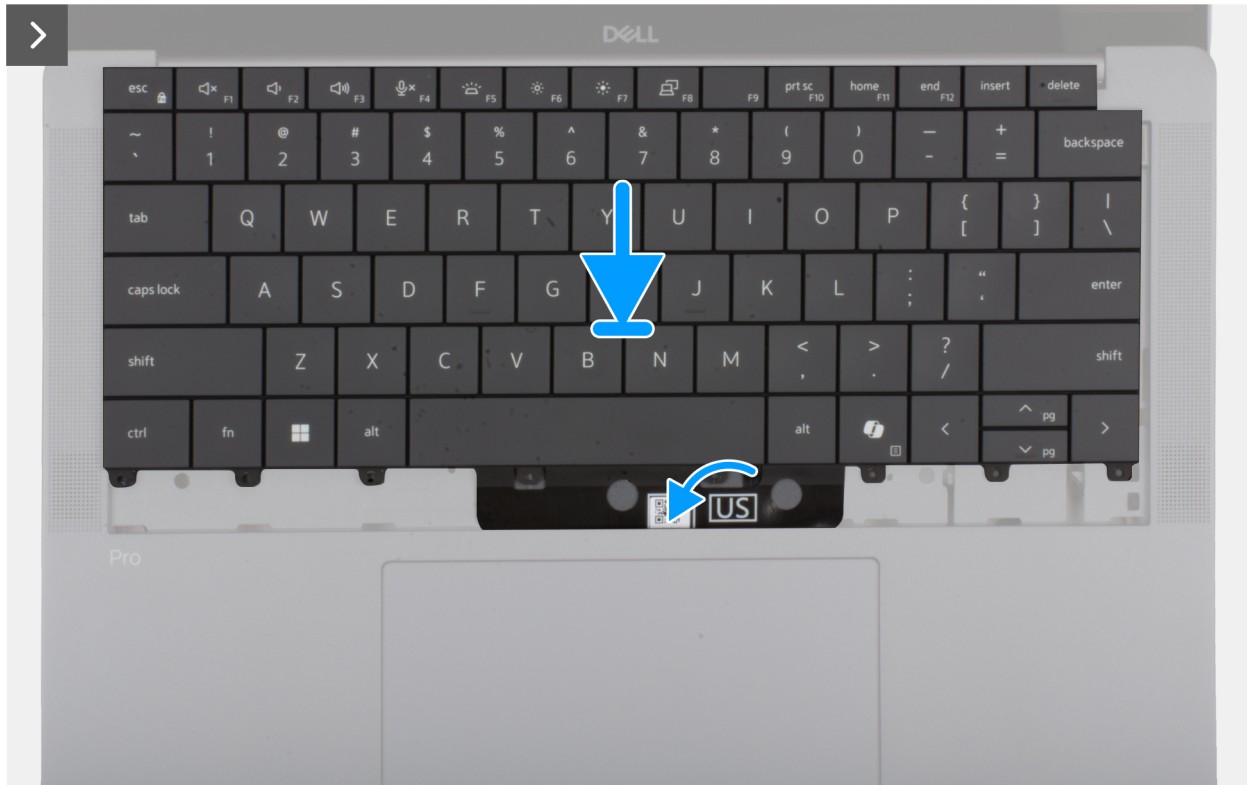
Figure 73. Installing the keyboard assembly
