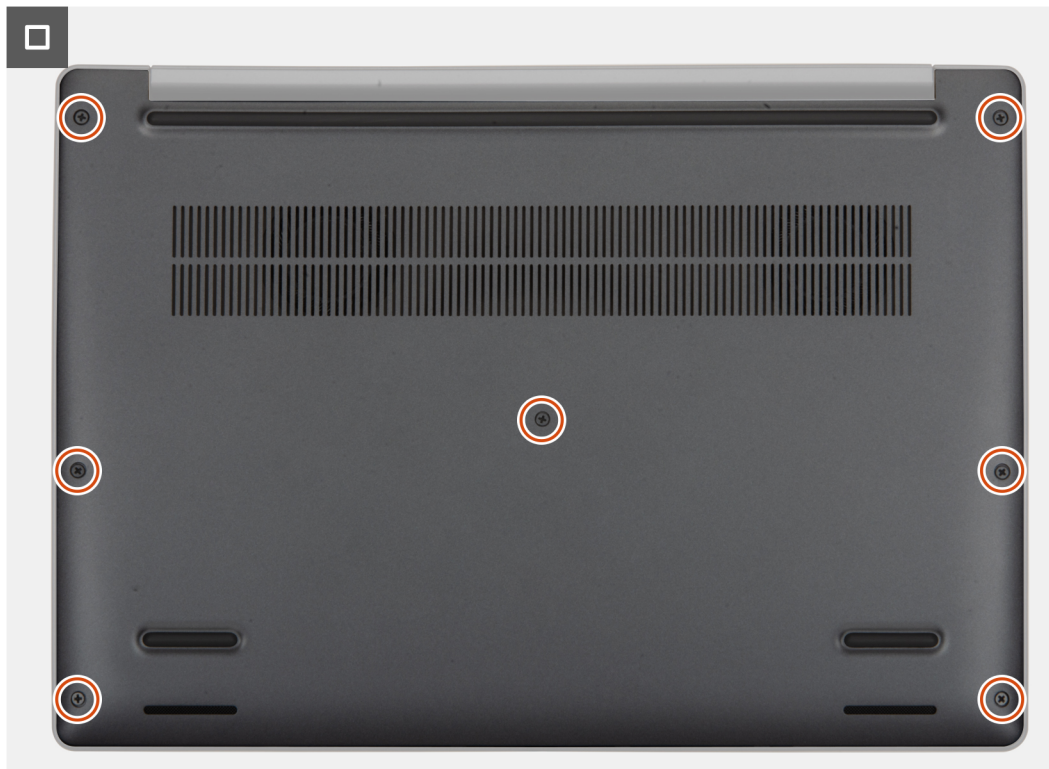
Figure 19. Tighten the captive screws
