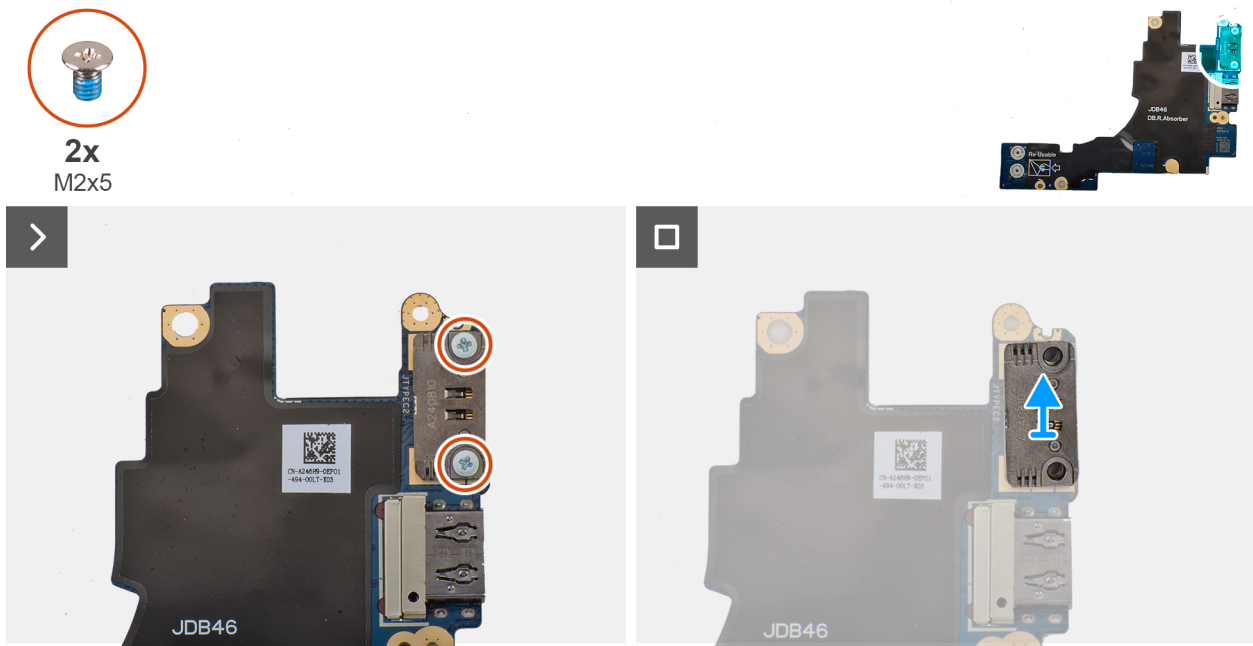
Figure 50. Removing the left USB Type-C module
