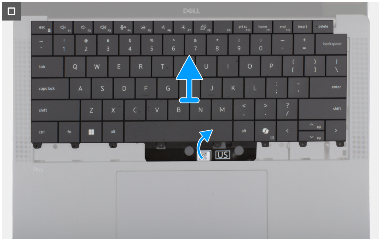
Figure 72. Removing the keyboard assembly
